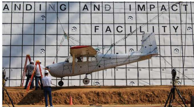
Figure 5. Pre-test photograph of C-172 crash Test 2 aircraft at impact attitude.
