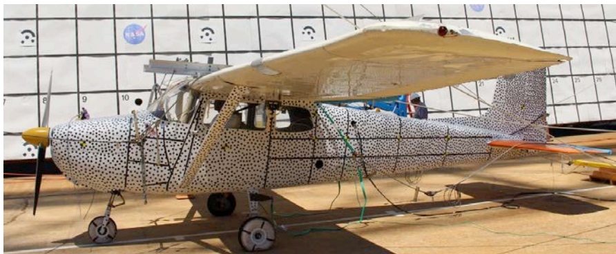
Figure 2. Pre-test photograph of C-172 crash Test 1.
