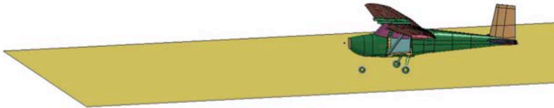
Figure A17. Case 3 model, straight tail aircraft impacting rigid surface at cruise velocity.
