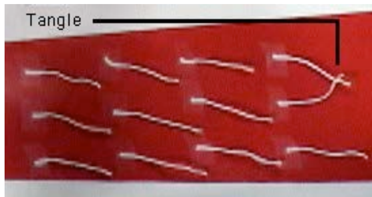
Picture 2. This does not represent the actual surface flow, but rather the result of two individual tufts getting tangled.
