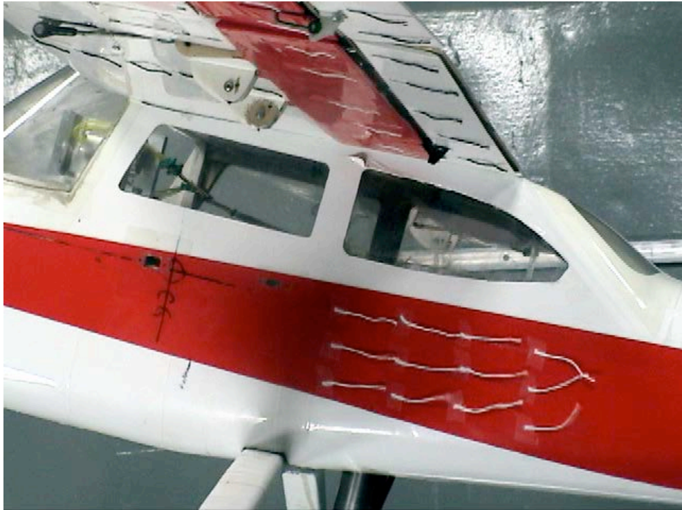
Figure C-114. Inboard and fuselage views; Aux-In-0_Aux-Out-0_Split-0_Ail-0; \alpha = 16^\circ .
