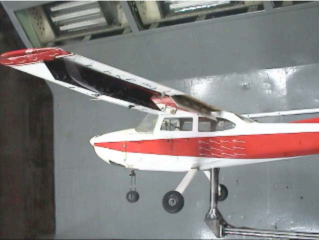
Figure C-166. Fuselage view; LSS-In-0_LSS-Out-45_Split-60_Ail-0; \alpha = 4^\circ .
