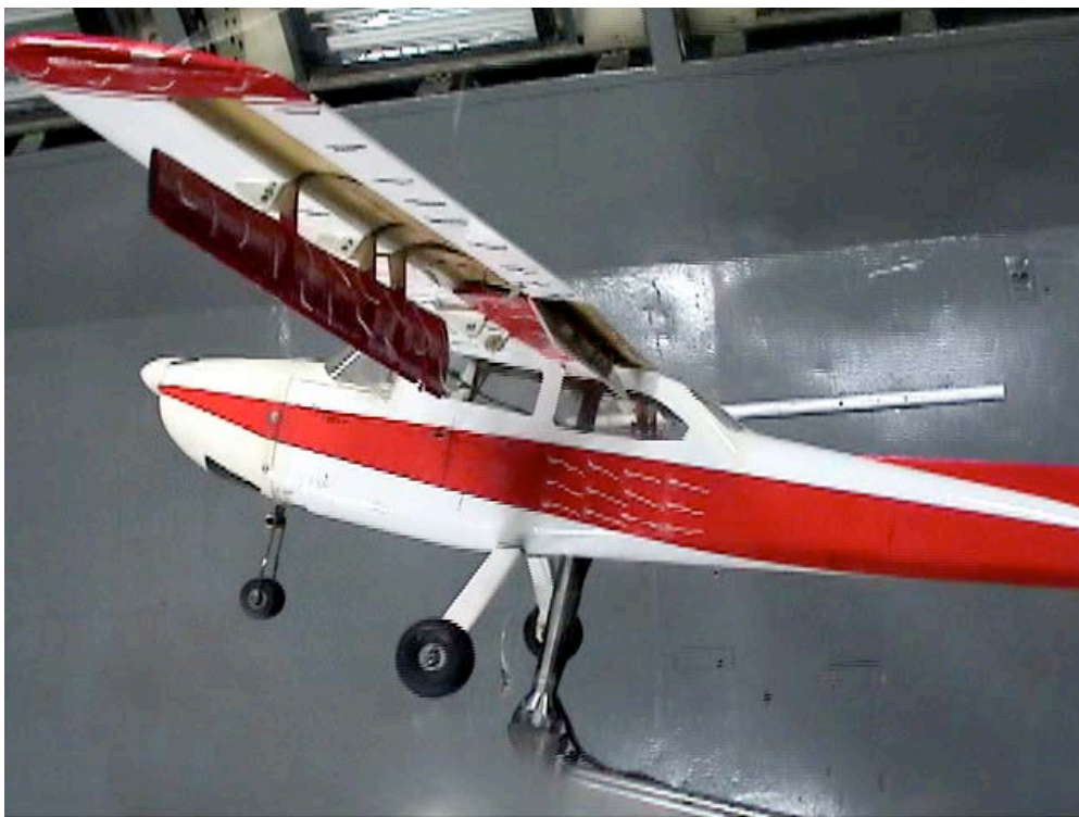
Figure C-62. Fuselage view; Aux-In-0_Aux-Out-90_Split-60_Ail-0; \alpha = 16^\circ .
