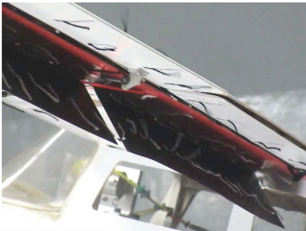
Figure C-145. Inboard view; LSS-In-45_LSS-Out-45_Split-0_Ail-0; \alpha = 16^\circ .
