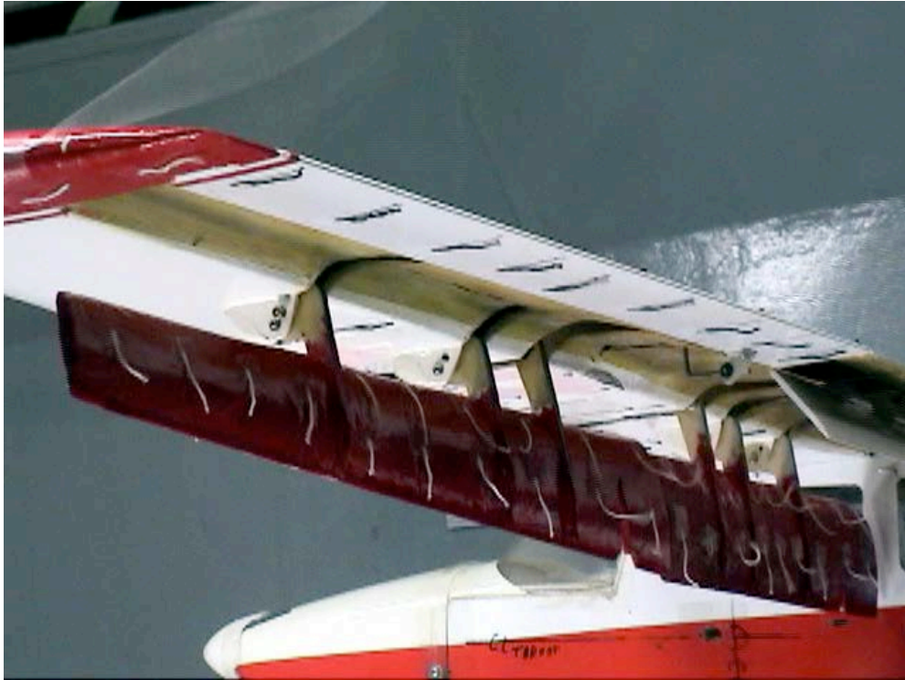
Figure C-67. Outboard tip view; Aux-In-90_Aux-Out-90_Split-60_Ail-0; \alpha = 4^\circ .
