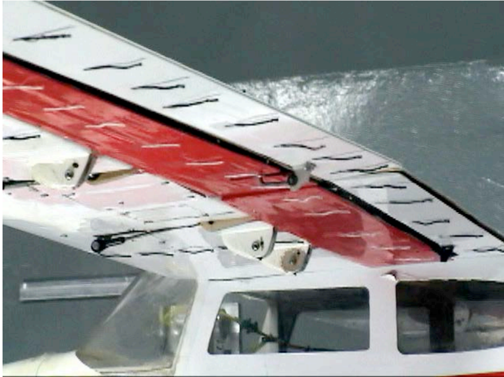
Figure C-103. Inboard view; Aux-In-0_Aux-Out-0_Split-0_Ail-0; \alpha = 0^\circ .
