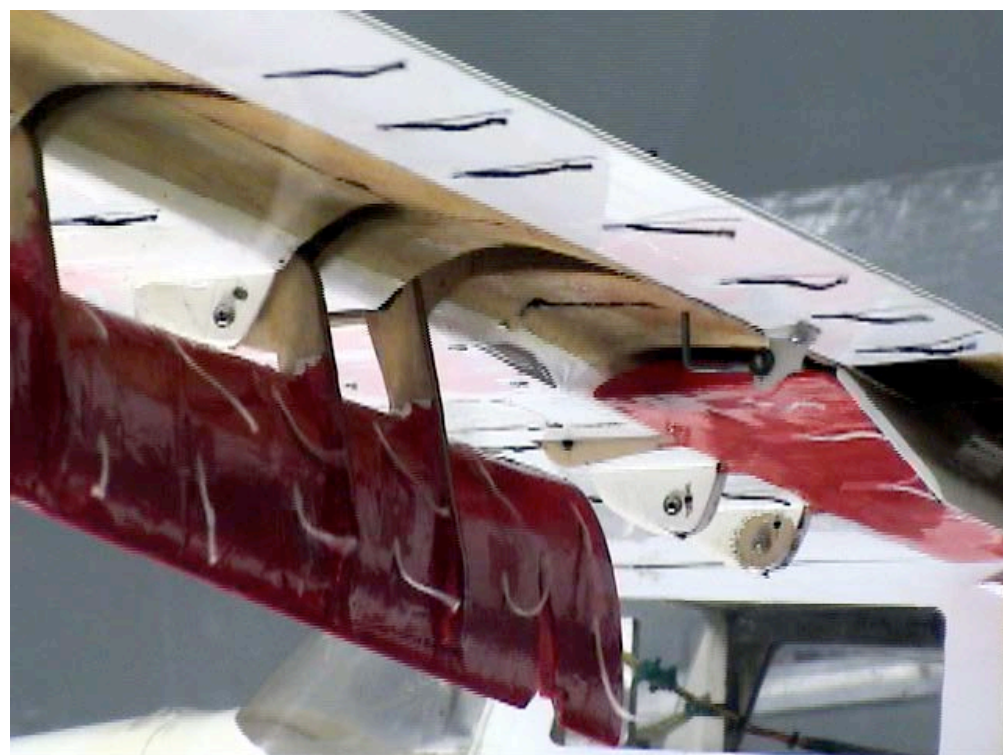
Figure C-54. Inboard view; Aux-In-0_Aux-Out-90_Split-60_Ail-0; \alpha = 8^\circ .
