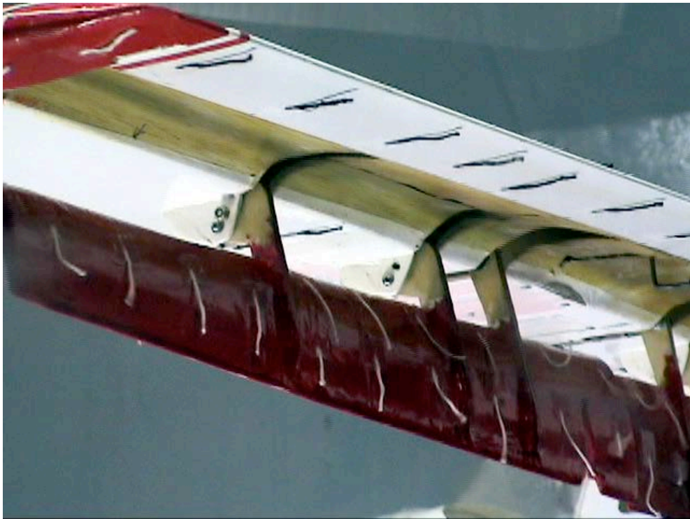
Figure C-64. Outboard tip view; Aux-In-90_Aux-Out-90_Split-60_Ail-0; \alpha = 0^\circ .
