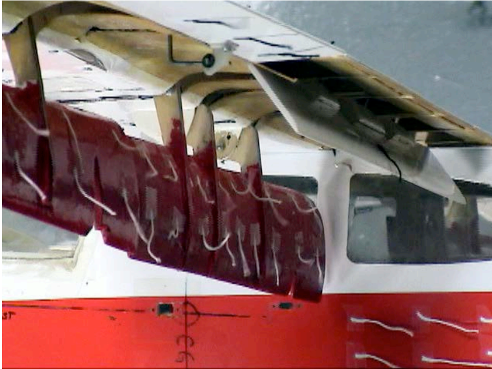
Figure C-69. Inboard view; Aux-In-90_Aux-Out-90_Split-60_Ail-0; \alpha = 8^\circ .
