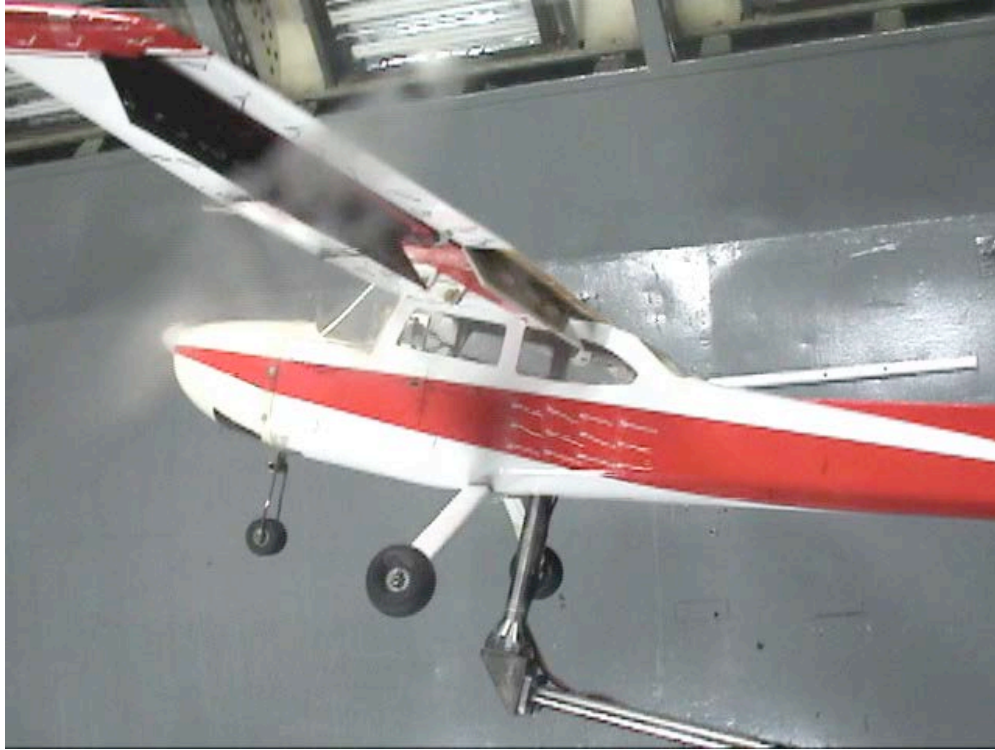
Figure C-175. Fuselage view; LSS-In-0_LSS-Out-45_Split-60_Ail-0; \alpha = 16^\circ .
