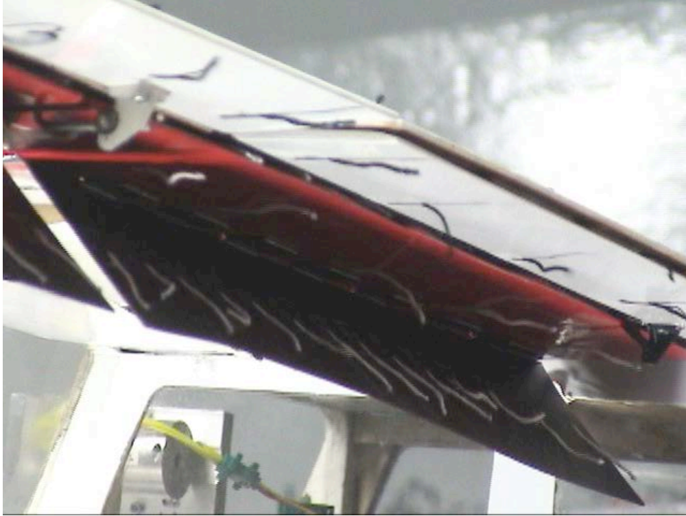
Figure C-139. Inboard view; LSS-In-45_LSS-Out-45_Split-0_Ail-0; \alpha = 8^\circ .
