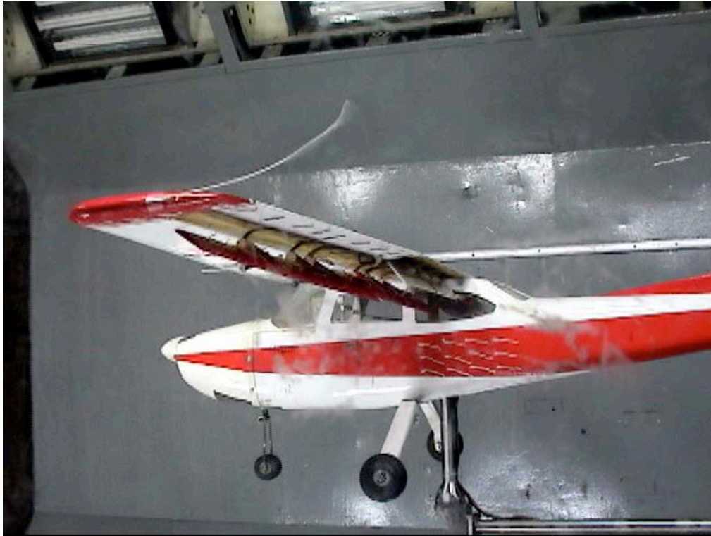
Figure C-3. Fuselage view; Aux-In-45_Aux-Out-45_Split-60_Ail-0; \alpha = 0^\circ .
