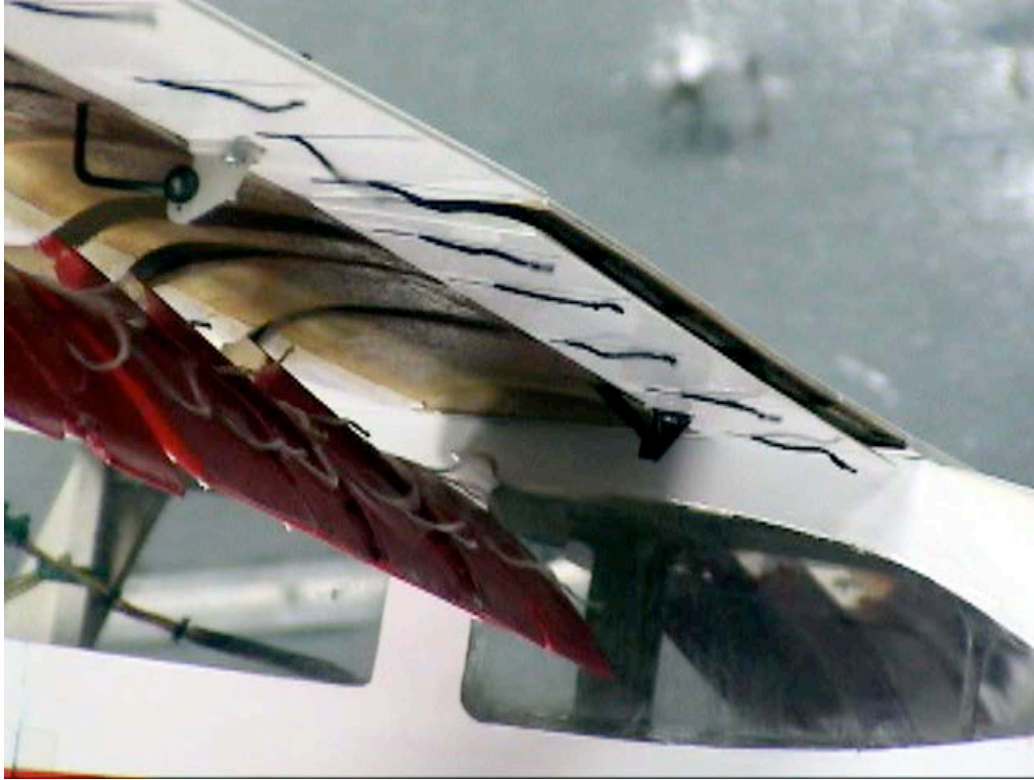
Figure C-27. Inboard view; Aux-In-45_Aux-Out-45_Split-0_Ail-0; \alpha = 12^\circ .
