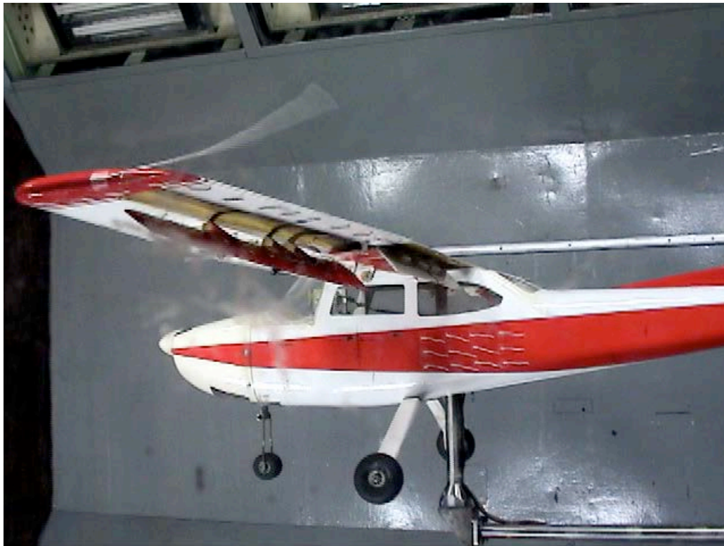
Figure C-35. Fuselage view; Aux-In-0_Aux-Out-45_Split-60_Ail-0; \alpha = 0^\circ .
