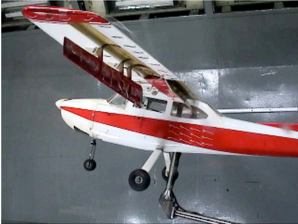
Figure C-59. Fuselage view; Aux-In-0_Aux-Out-90_Split-60_Ail-0; \alpha = 12^\circ .
