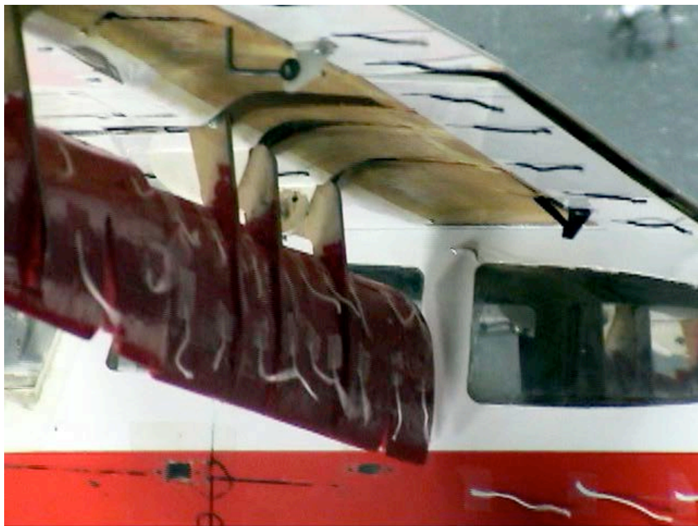
Figure C-84. Inboard view; Aux-In-90_Aux-Out-90_Split-0_Ail-0; \alpha = 8^\circ .
