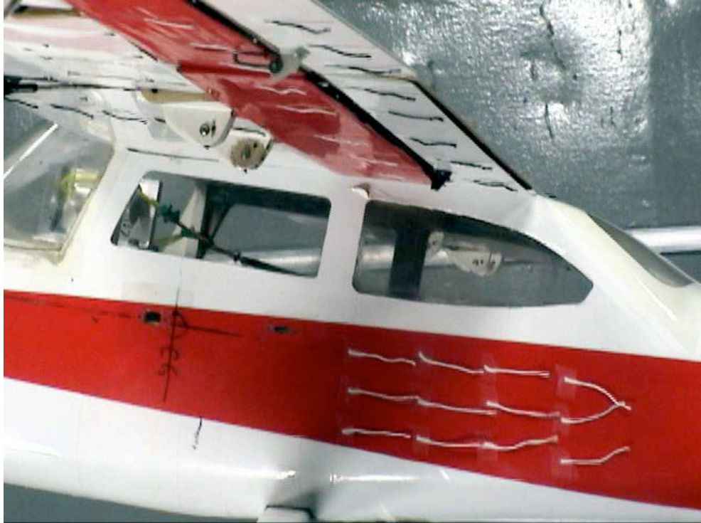
Figure C-111. Inboard view; Aux-In-0_Aux-Out-0_Split-0_Ail-0; \alpha = 12^\circ .
