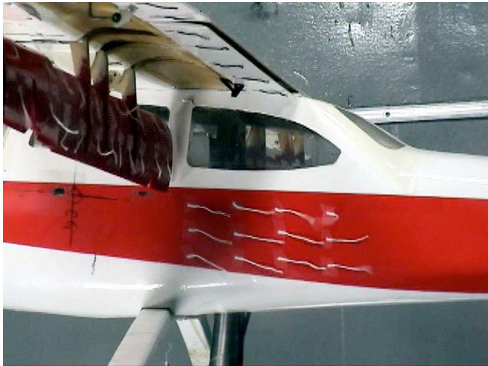
Figure C-86. Fuselage view; Aux-In-90_Aux-Out-90_Split-0_Ail-0; \alpha = 8^\circ .
