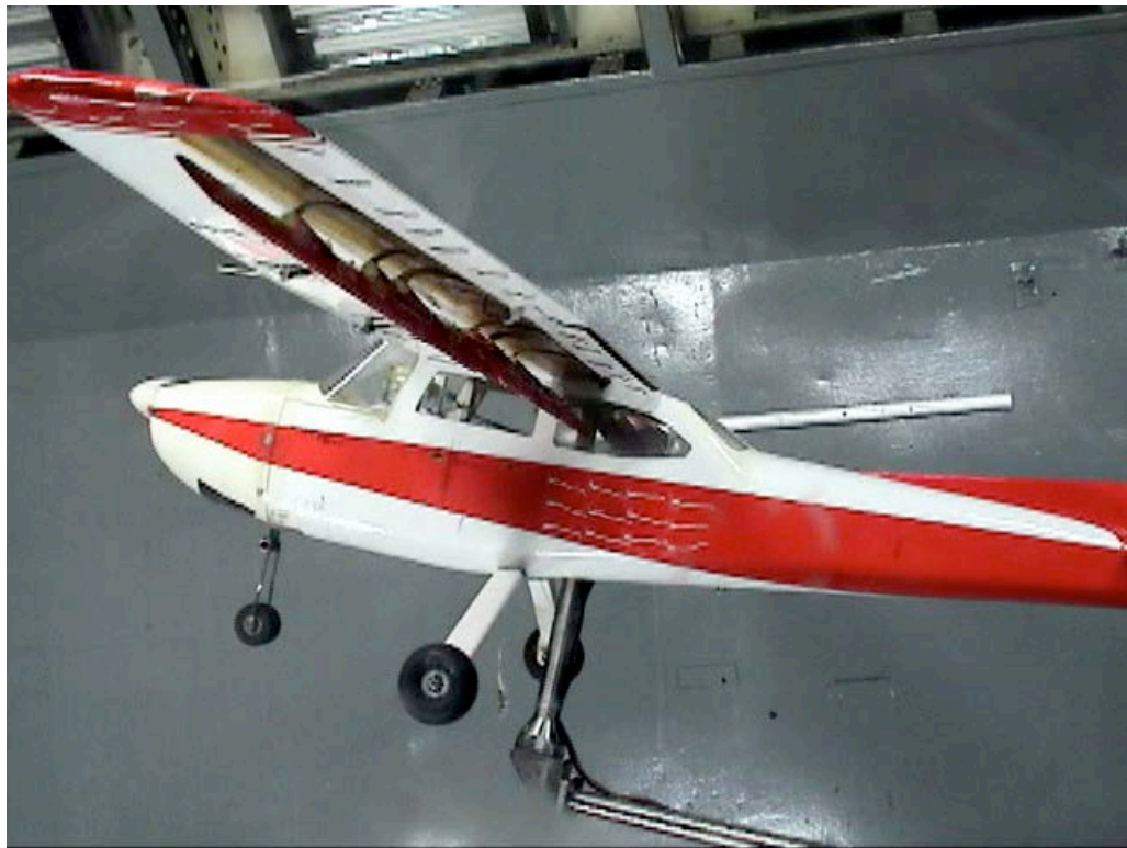
Figure C-32. Fuselage view; Aux-In-45_Aux-Out-45_Split-0_Ail-0; \alpha = 16^\circ .
