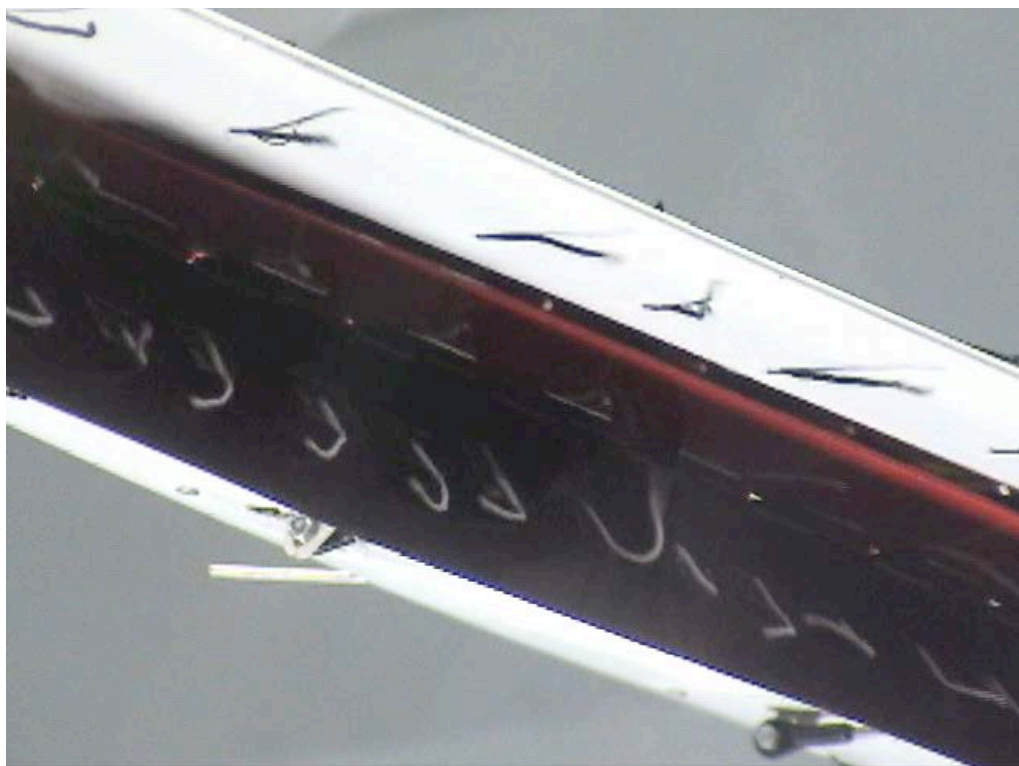
Figure C-158. Outboard tip view; LSS-In-0_LSS-Out-45_Split-0_Ail-0; \alpha = 12^\circ .
