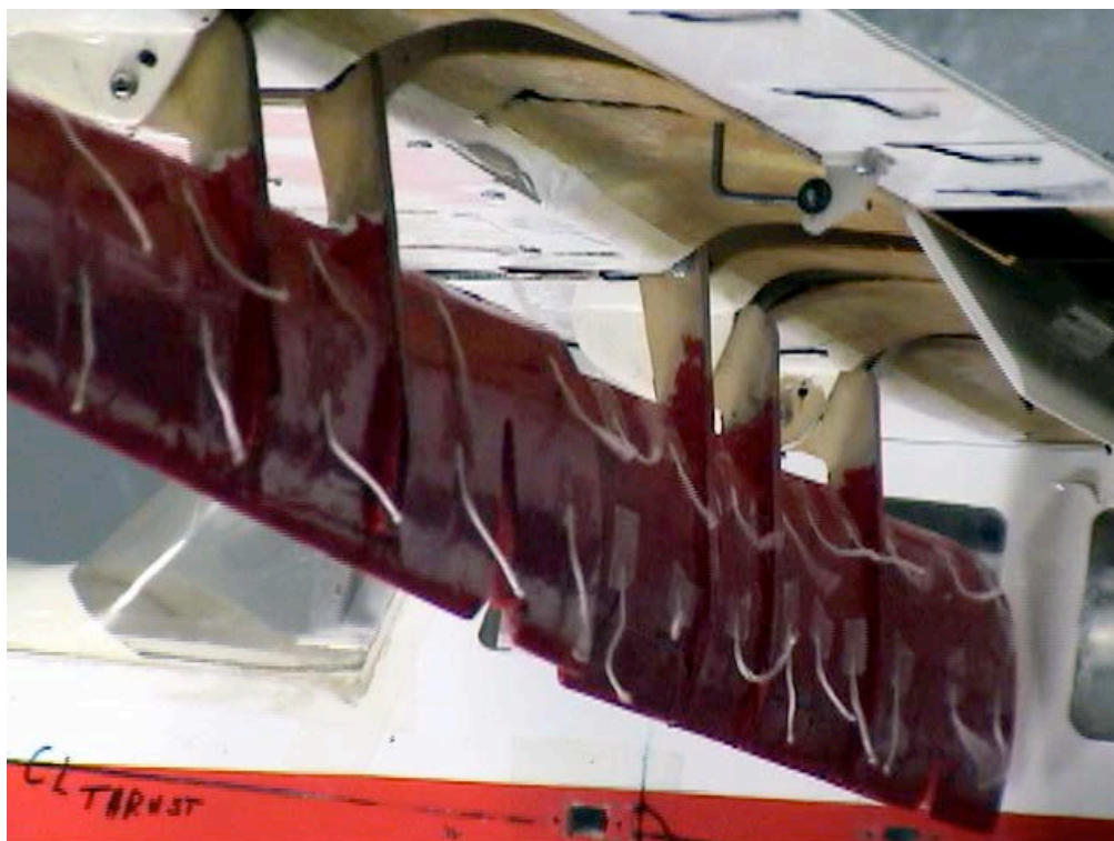
Figure C-73. Outboard tip view; Aux-In-90_Aux-Out-90_Split-60_Ail-0; \alpha = 12^\circ .
