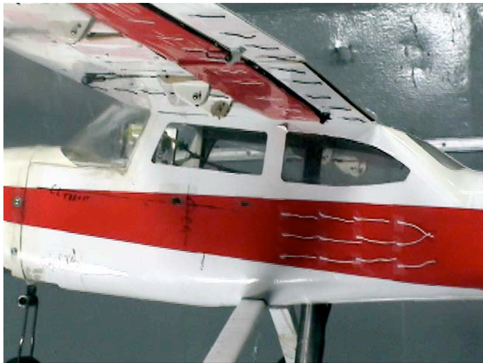
Figure C-108. Inboard view; Aux-In-0_Aux-Out-0_Split-0_Ail-0; \alpha = 8^\circ .
