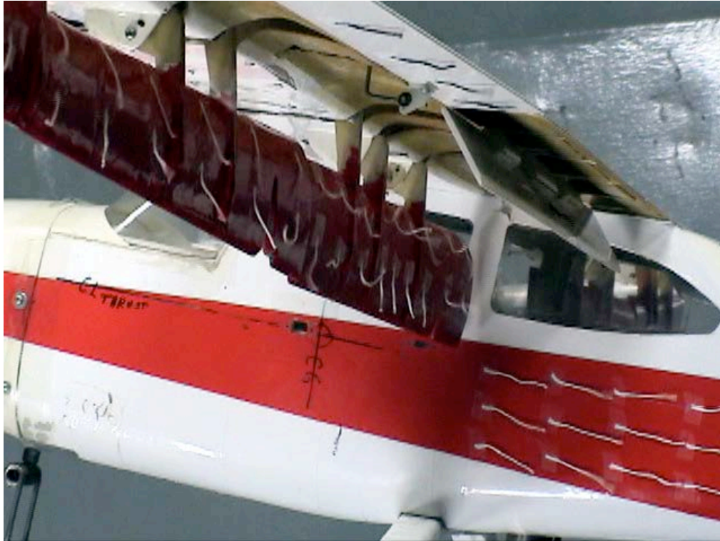
Figure C-75. Inboard view; Aux-In-90_Aux-Out-90_Split-60_Ail-0; \alpha = 16^\circ .
