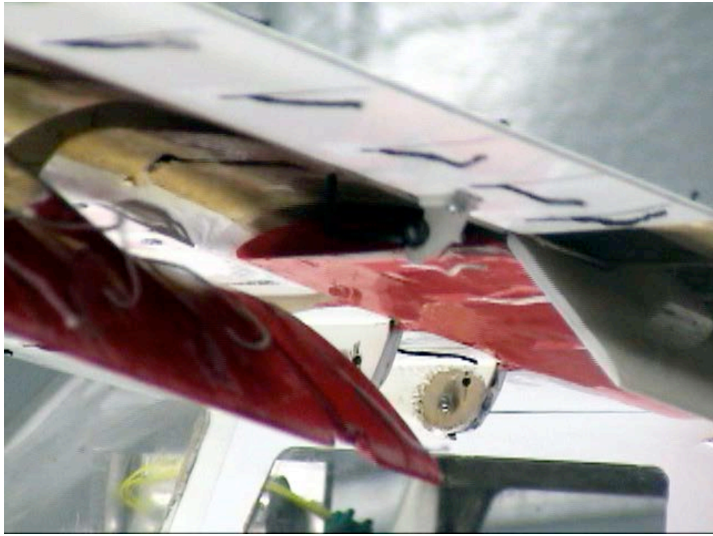
Figure C-39. Inboard view; Aux-In-0_Aux-Out-45_Split-60_Ail-0; \alpha = 8^\circ .
