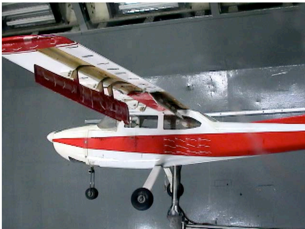
Figure C-53. Fuselage view; Aux-In-0_Aux-Out-90_Split-60_Ail-0; \alpha = 4^\circ .
