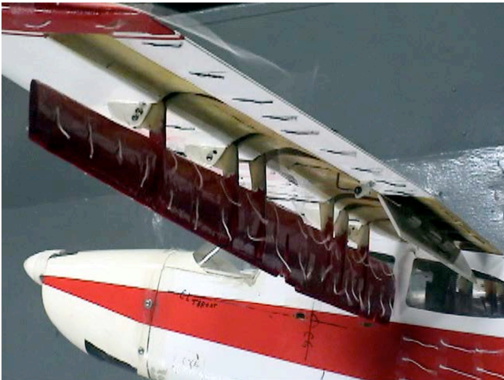
Figure C-76. Outboard tip view; Aux-In-90_Aux-Out-90_Split-60_Ail-0; \alpha = 16^\circ .
