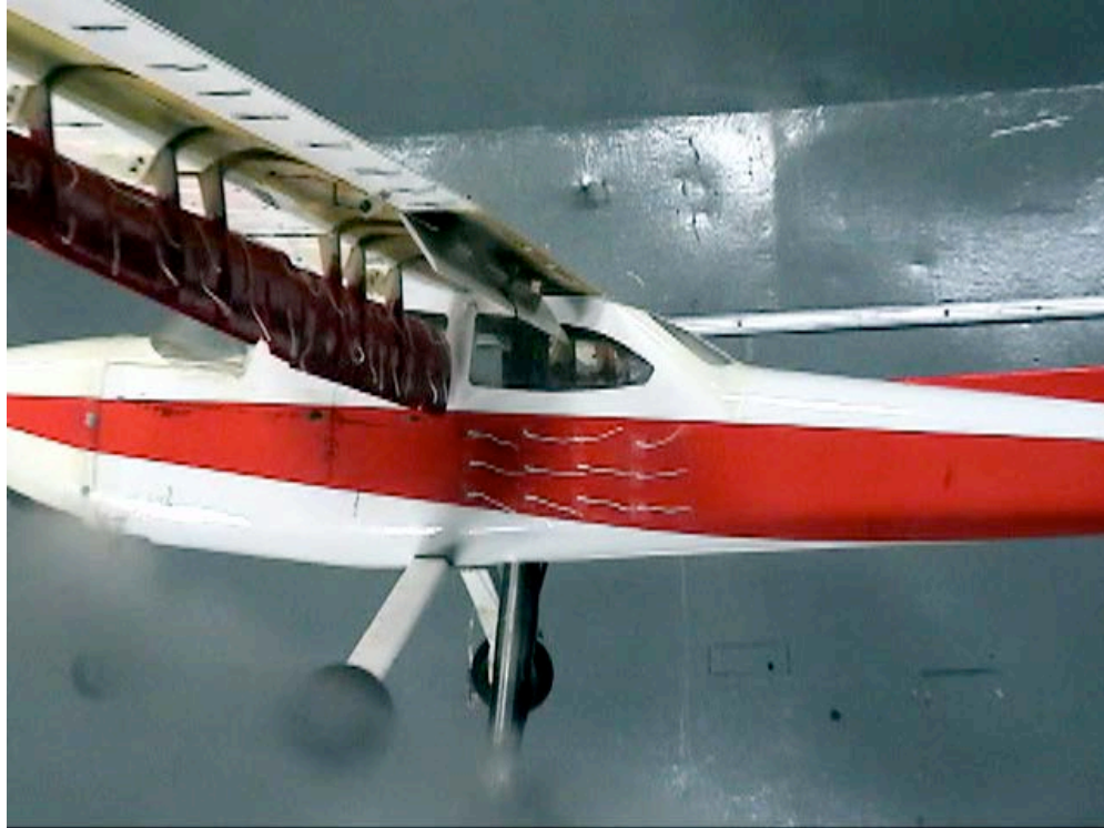
Figure C-71. Fuselage view; Aux-In-90_Aux-Out-90_Split-60_Ail-0; \alpha = 8^\circ .
