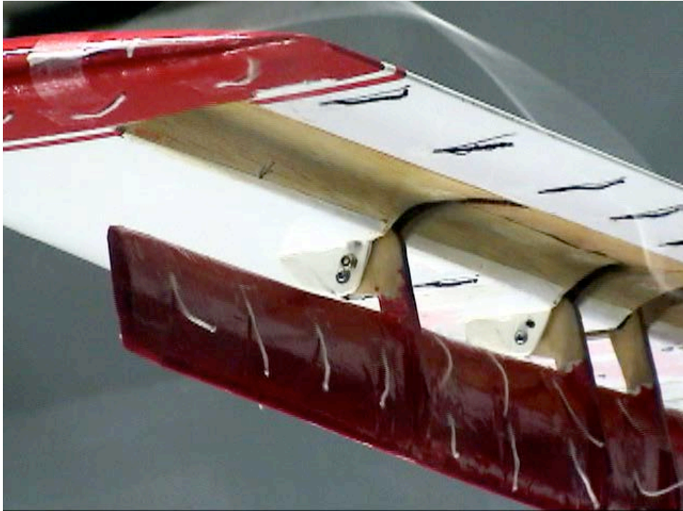
Figure C-55. Outboard tip view; Aux-In-0_Aux-Out-90_Split-60_Ail-0; \alpha = 8^\circ .
