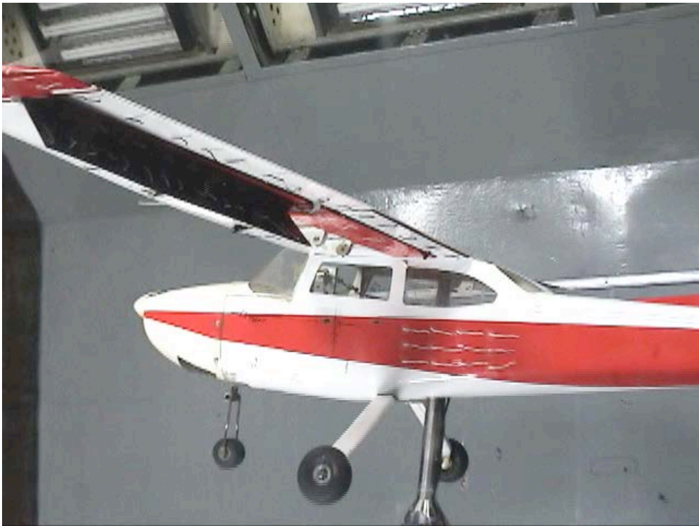
Figure C-156. Fuselage view; LSS-In-0_LSS-Out-45_Split-0_Ail-0; \alpha = 8^\circ .
