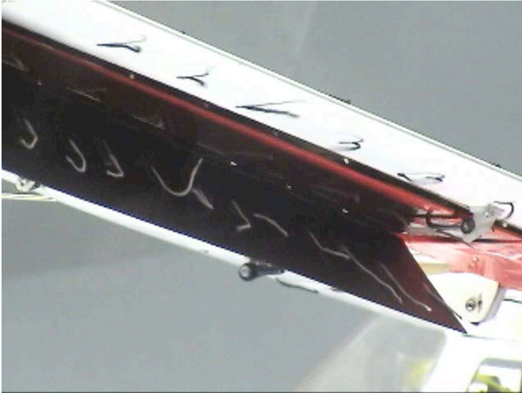
Figure C-157. Inboard view; LSS-In-0_LSS-Out-45_Split-0_Ail-0; \alpha = 12^\circ .
