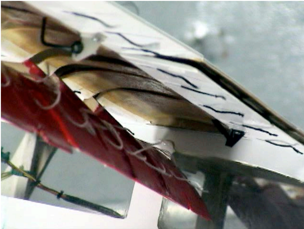
Figure C-30. Inboard view; Aux-In-45_Aux-Out-45_Split-0_Ail-0; \alpha = 16^\circ .
