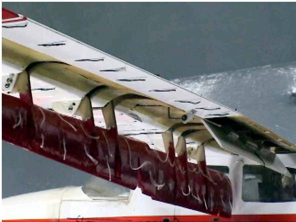
Figure C-70. Outboard tip view; Aux-In-90_Aux-Out-90_Split-60_Ail-0; \alpha = 8^\circ .
