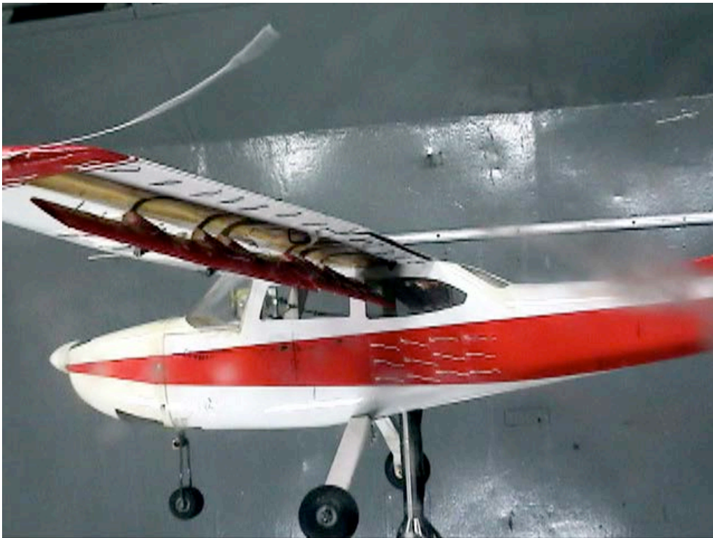
Figure C-20. Fuselage view; Aux-In-45_Aux-Out-45_Split-0_Ail-0; \alpha = 0^\circ .
