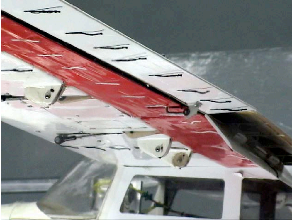
Figure C-95. Inboard view; Aux-In-0_Aux-Out-0_Split-60_Ail-0; \alpha = 4^\circ .
