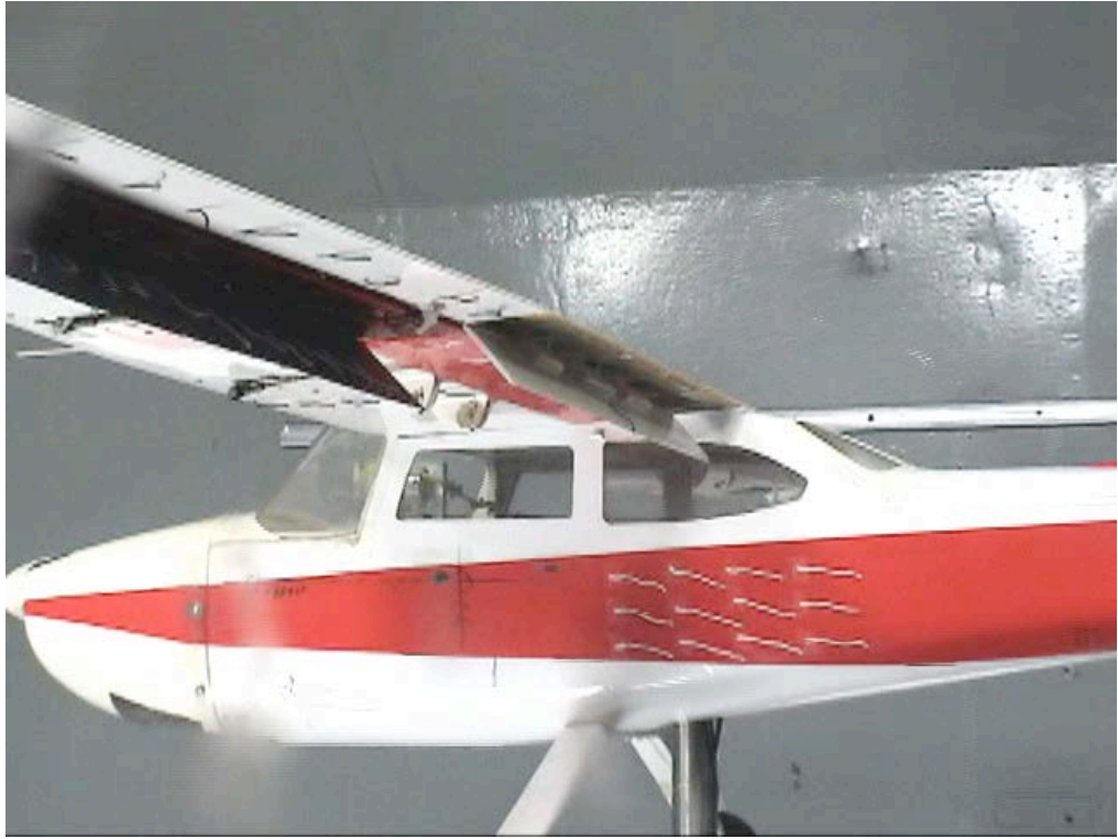
Figure C-164. Fuselage view; LSS-In-0_LSS-Out-45_Split-60_Ail-0; \alpha = 0^\circ .
