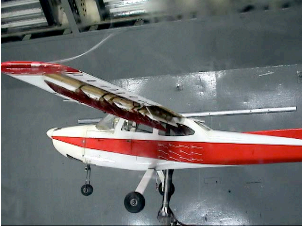
Figure C-9. Fuselage view; Aux-In-45_Aux-Out-45_Split-60_Ail-0; \alpha = 8^\circ .
