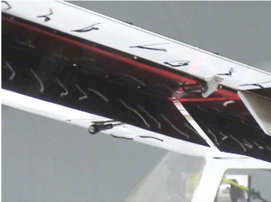
Figure C-124. Mid-span view; LSS-In-45_LSS-Out-45_Split-60_Ail-0; \alpha = 8^\circ .
