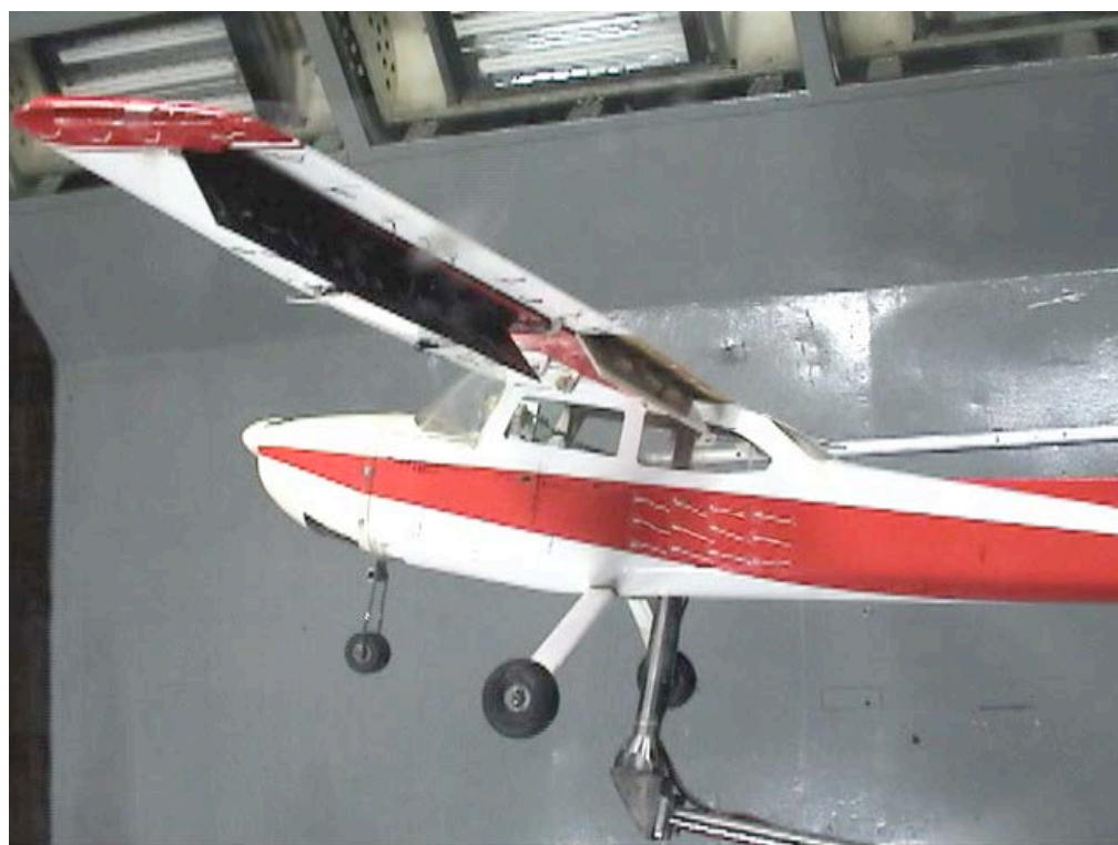
Figure C-172. Fuselage view; LSS-In-0_LSS-Out-45_Split-60_Ail-0; \alpha = 12^\circ .
