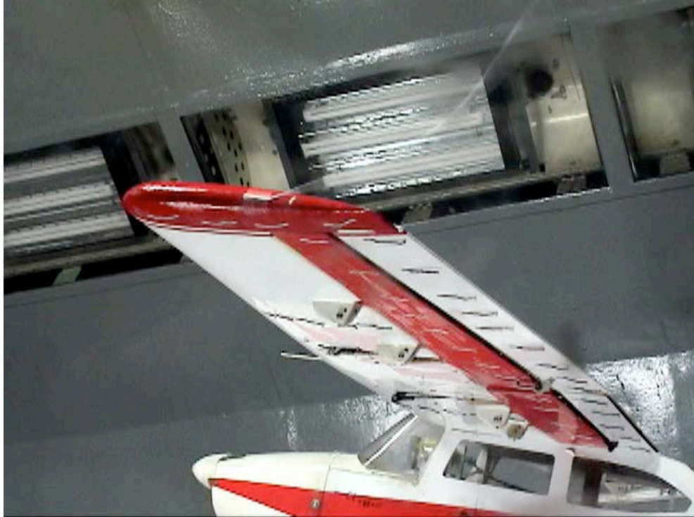
Figure C-115. Outboard tip view; Aux-In-0_Aux-Out-0_Split-0_Ail-0; \alpha = 16^\circ .
