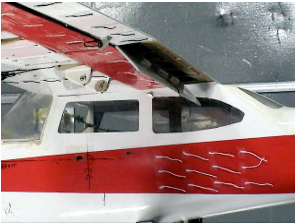
Figure C-94. Fuselage view; Aux-In-0_Aux-Out-0_Split-60_Ail-0; \alpha = 0^\circ .
