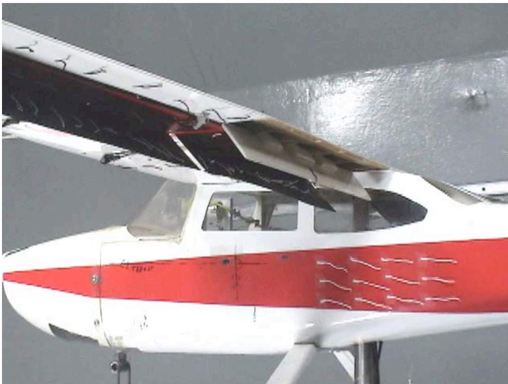
Figure C-122. Fuselage view; LSS-In-45_LSS-Out-45_Split-60_Ail-0; \alpha = 4^\circ .
