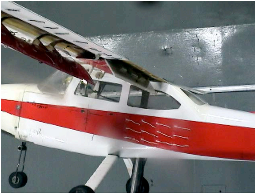
Figure C-44. Fuselage view; Aux-In-0_Aux-Out-45_Split-60_Ail-0; \alpha = 12^\circ .
