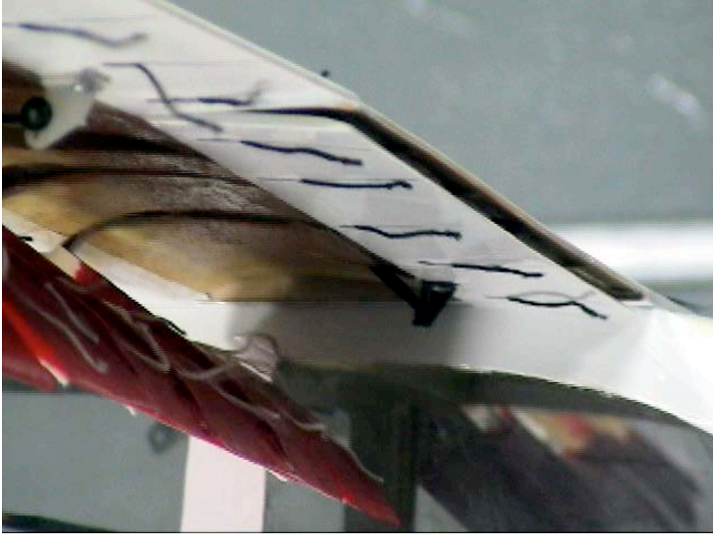
Figure C-21. Inboard view; Aux-In-45_Aux-Out-45_Split-0_Ail-0; \alpha = 4^\circ .
