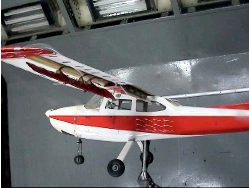
Figure C-41. Fuselage view; Aux-In-0_Aux-Out-45_Split-60_Ail-0; \alpha = 8^\circ .
