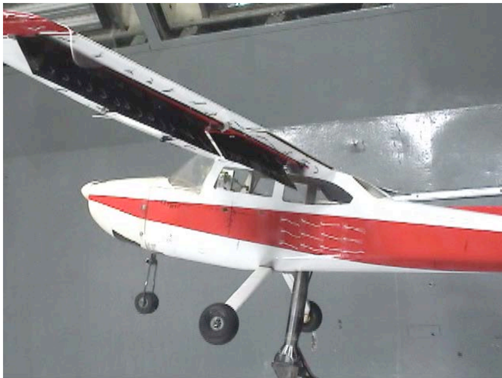
Figure C-144. Fuselage view; LSS-In-45_LSS-Out-45_Split-0_Ail-0; \alpha = 12^\circ .
