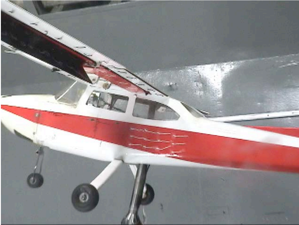
Figure C-161. Fuselage view; LSS-In-0_LSS-Out-45_Split-0_Ail-0; \alpha = 16^\circ .
