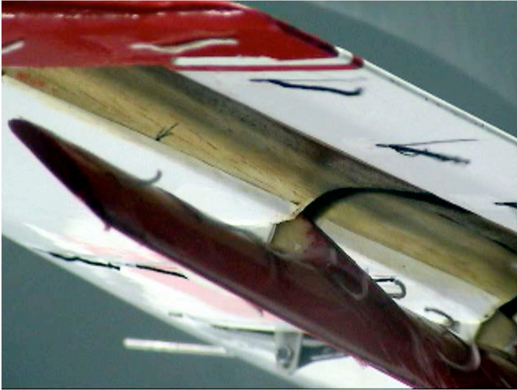
Figure C-31. Outboard tip view; Aux-In-45_Aux-Out-45_Split-0_Ail-0; \alpha = 16^\circ .
