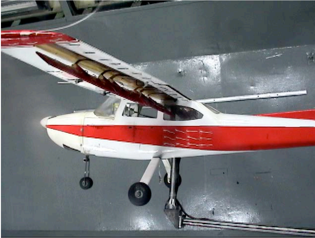
Figure C-26. Fuselage view; Aux-In-45_Aux-Out-45_Split-0_Ail-0; \alpha = 8^\circ .
