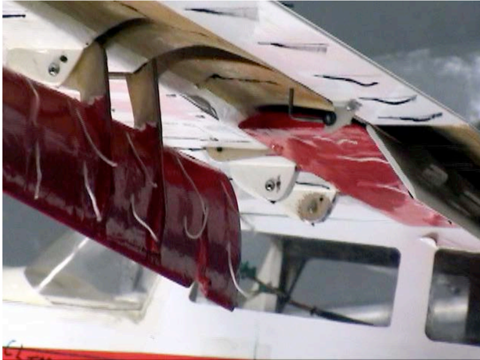
Figure C-57. Inboard view; Aux-In-0_Aux-Out-90_Split-60_Ail-0; \alpha = 12^\circ .
