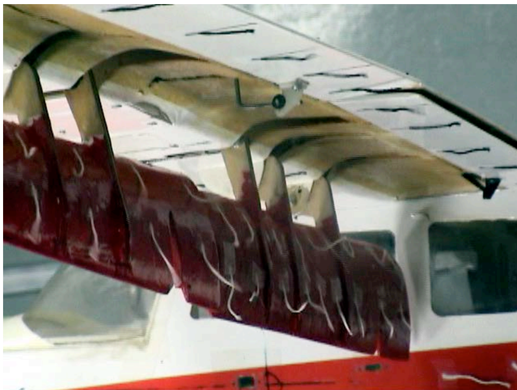
Figure C-81. Inboard view; Aux-In-90_Aux-Out-90_Split-0_Ail-0; \alpha = 4^\circ .
