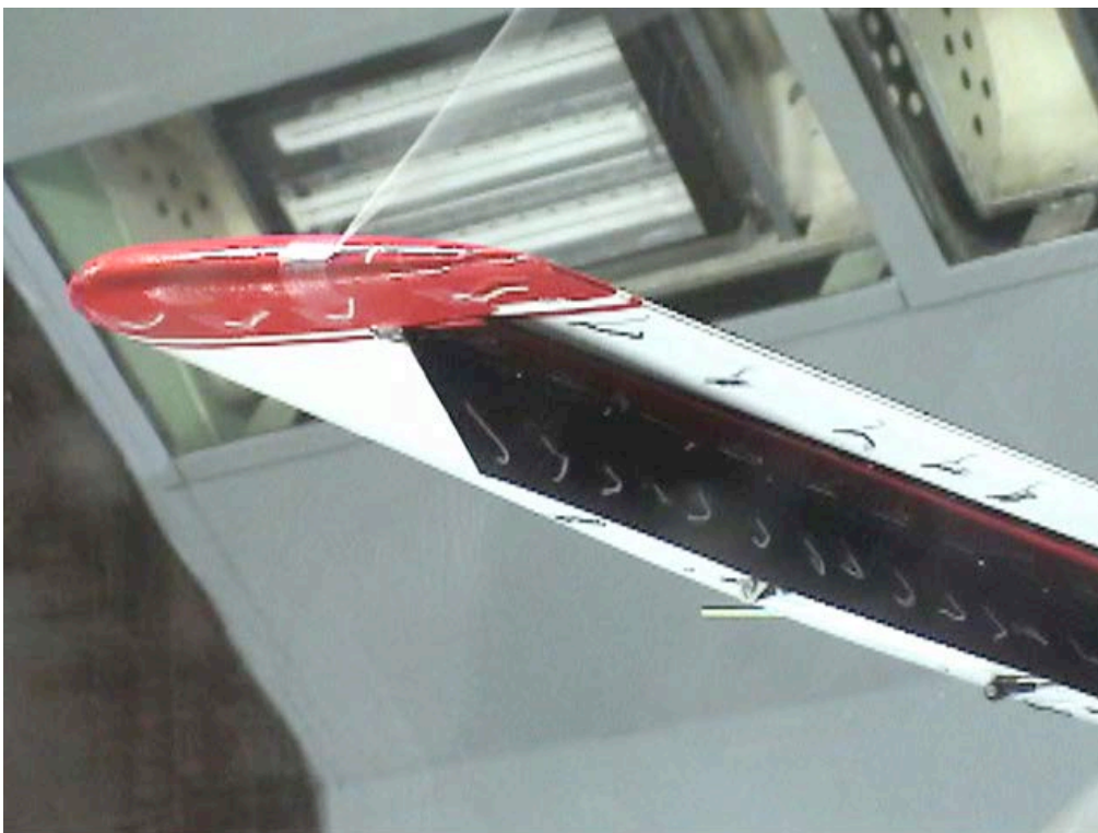
Figure C-128. Outboard tip view; LSS-In-45_LSS-Out-45_Split-60_Ail-0; \alpha = 12^\circ .
