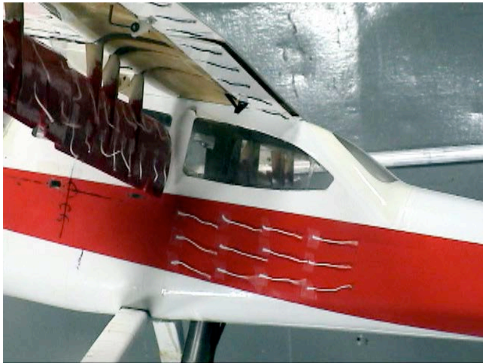
Figure C-92. Fuselage view; Aux-In-90_Aux-Out-90_Split-0_Ail-0; \alpha = 16^\circ .
