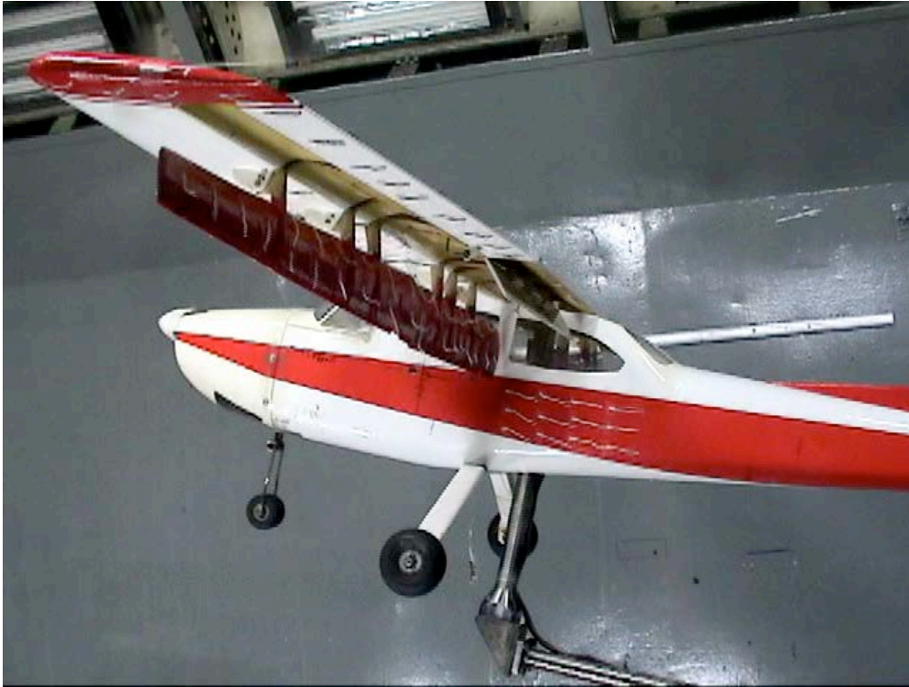
Figure C-77. Fuselage view; Aux-In-90_Aux-Out-90_Split-60_Ail-0; \alpha = 16^\circ .
