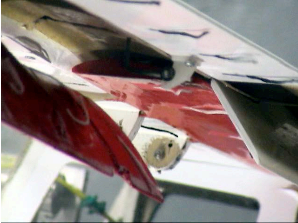
Figure C-45. Inboard view; Aux-In-0_Aux-Out-45_Split-60_Ail-0; \alpha = 16^\circ .
