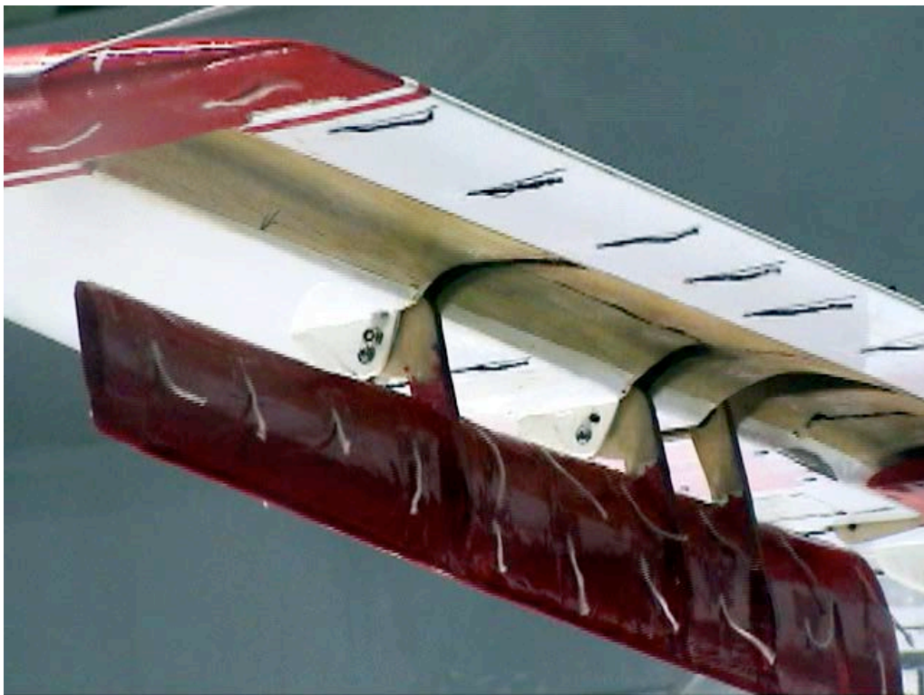
Figure C-52. Outboard tip view; Aux-In-0_Aux-Out-90_Split-60_Ail-0; \alpha = 4^\circ .
