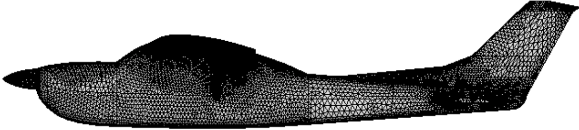
Figure B-1. Computational grid definition of aircraft.
