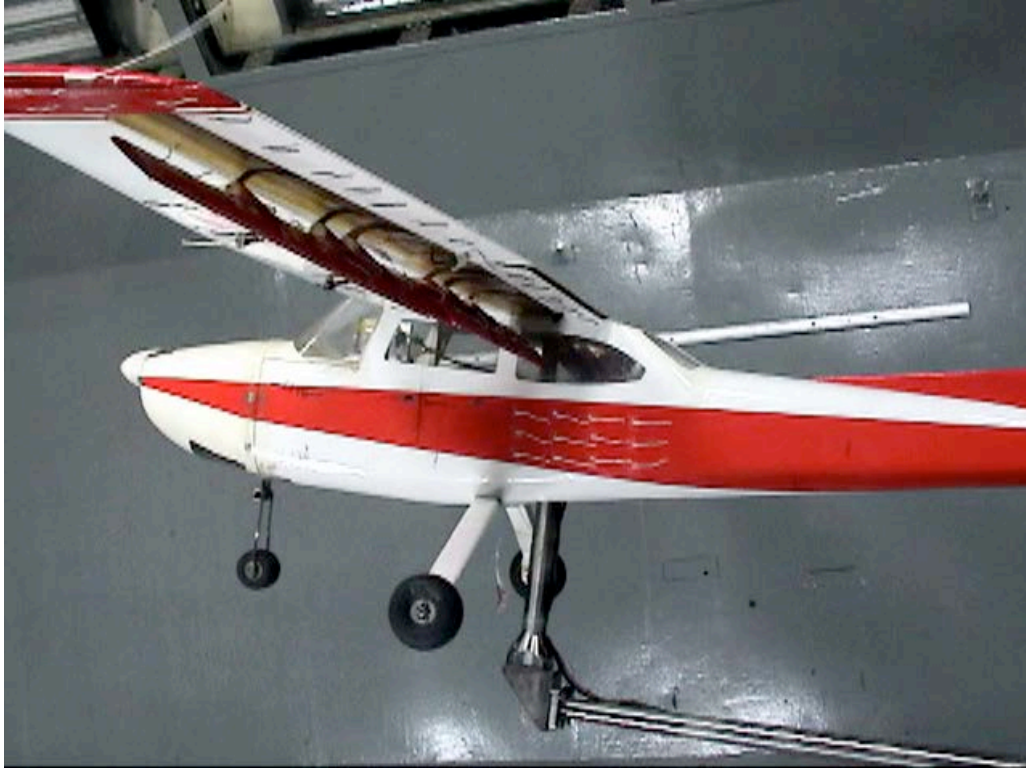
Figure C-29. Fuselage view; Aux-In-45_Aux-Out-45_Split-0_Ail-0; \alpha = 12^\circ .
