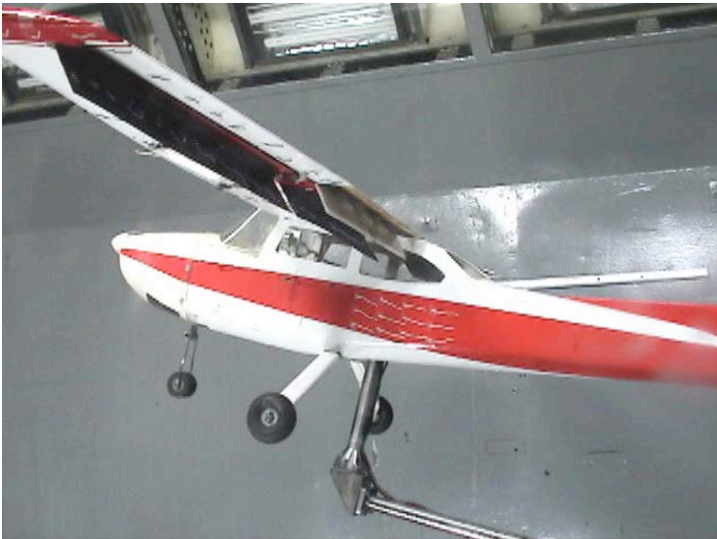
Figure C-132. Fuselage view; LSS-In-45_LSS-Out-45_Split-60_Ail-0; \alpha = 16^\circ .
