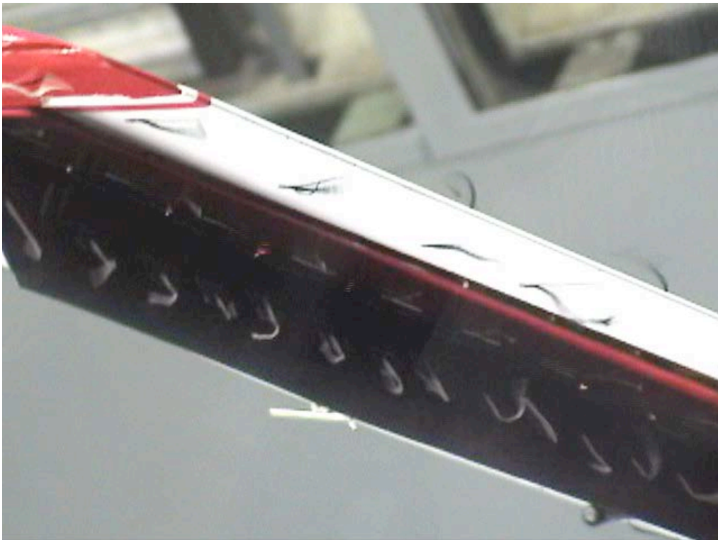
Figure C-160. Outboard tip view; LSS-In-0_LSS-Out-45_Split-0_Ail-0; \alpha = 16^\circ .
