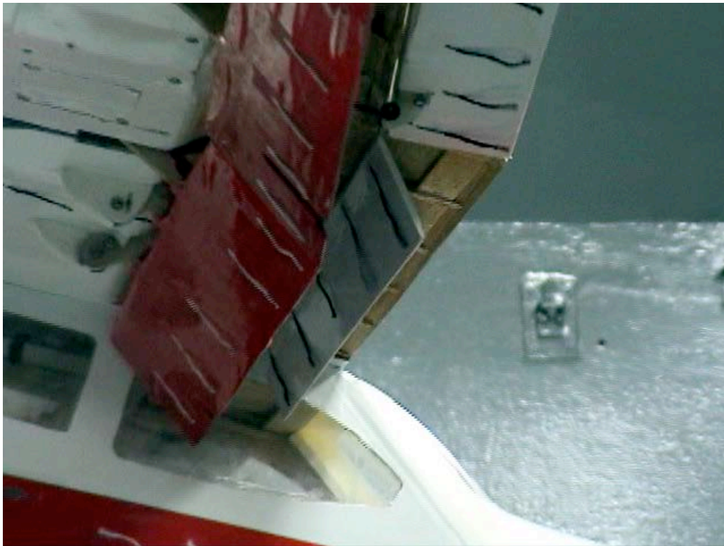
Figure C-16. Inboard lower surface view; Aux-In-45_Aux-Out-45_Split-60_Ail-0; \alpha = 16^\circ .
