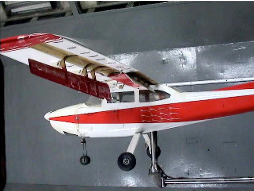
Figure C-50. Fuselage view; Aux-In-0_Aux-Out-90_Split-60_Ail-0; \alpha = 0^\circ .
