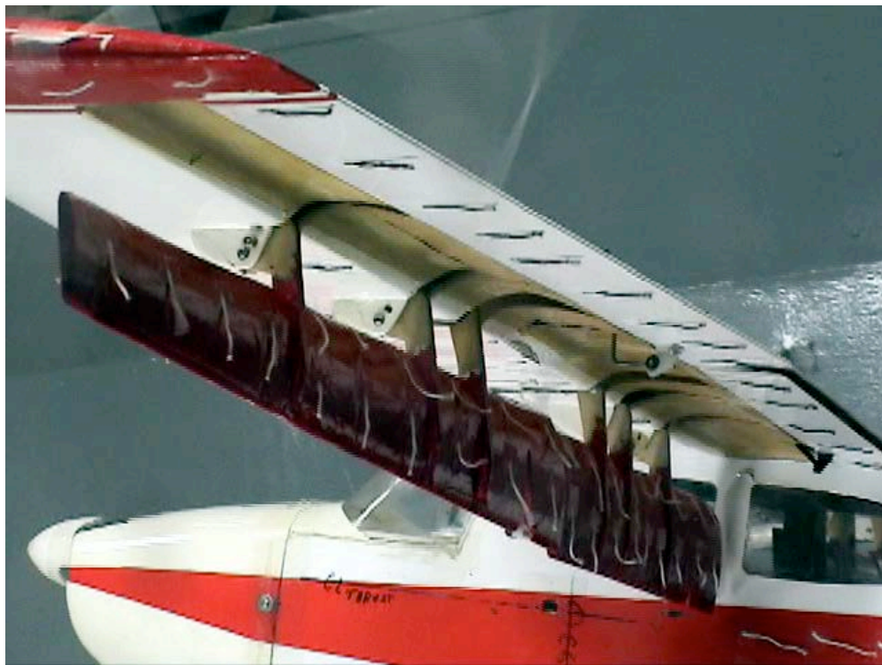
Figure C-88. Outboard tip view; Aux-In-90_Aux-Out-90_Split-0_Ail-0; \alpha = 12^\circ .
