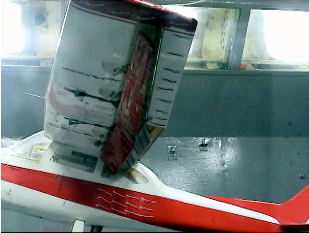
Figure C-17. Outboard lower surface view; Aux-In-45_Aux-Out-45_Split-60_Ail-0; \alpha = 16^\circ .
