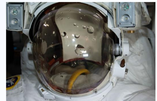
Extravehicular Mobility Unit (EMU) With Water in Helmet During Post-EVA 23 Screening Test
