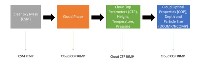
Figure 2: Simple schematic of the cloud product algorithm chain. The associated cloud RIMPs are below the algorithm/product, and the products are combined consistent with the algorithms that product them.
