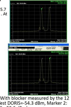
September 22<sup>nd</sup> : With blocker measured by the 1 meter(Marker 1:Test DORIS=-54.3 dBm, Marker 2 Operational DORIS=-50.6 dBm)
