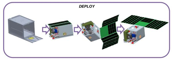
•Deployable solar arrays for power production
