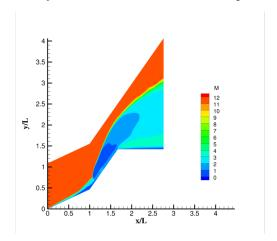
Figure 9. Computed Mach number contours for the Mach 11.3 flow over the CUBRC 15-25 double cone.
