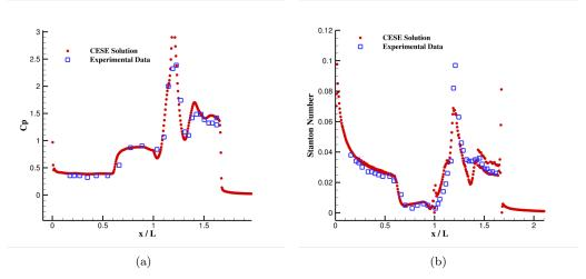
Figure 10. Comparison of computed surface pressure coffeicent and Stanton number with experimental data for the Mach 11.3 flow over a double cone: (a)  $C_p$  (b) Stanton number.
