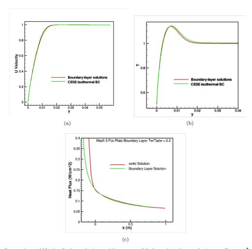
Figure 7. Comparison of Navier-Stokes solutions with compressible boundary-layer solutions at Re =  $10^5$  for a Mach 3 flate-plate flow with  $T_{wall,adiabatic} = 0.2$ : (a) streamwise velocity (non-dimensionalized by  $u_{\infty}$ ) (b) temperature (non-dimensionalized by  $T_{\infty}$ ) and (c) heat flux distribution along the streamwise direction.
