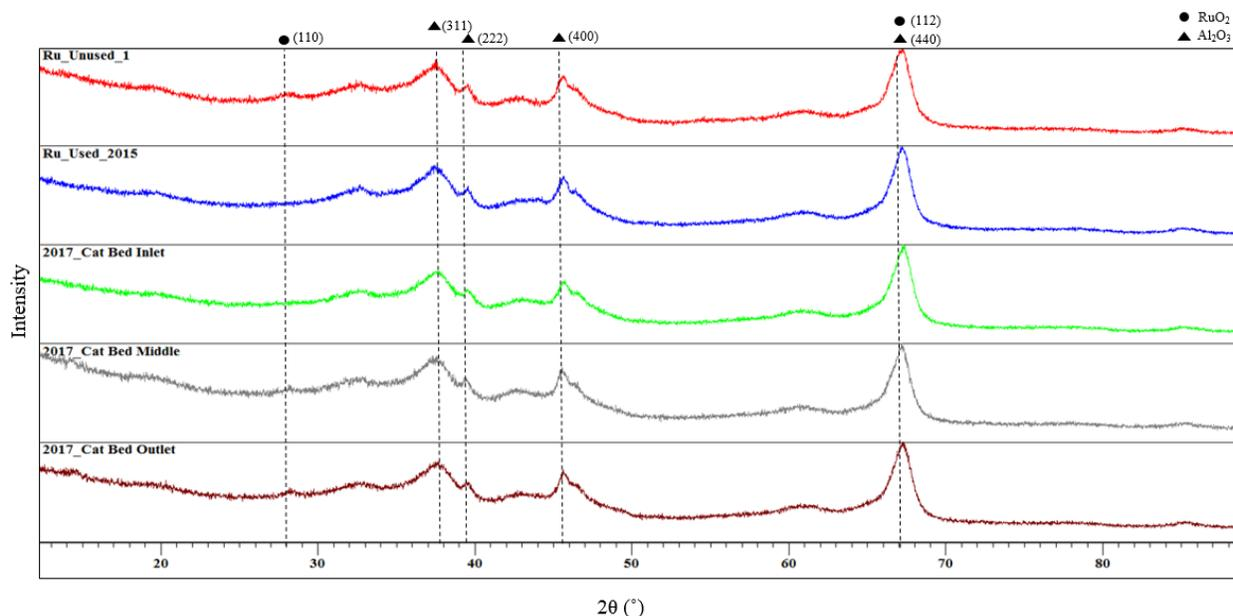
Figure 14. XRD Spectrums of Ru/Al<sub>2</sub>O<sub>3</sub> pellets from APM project, unused, used in 2015 (damaged), and used 2017 (not damaged).
