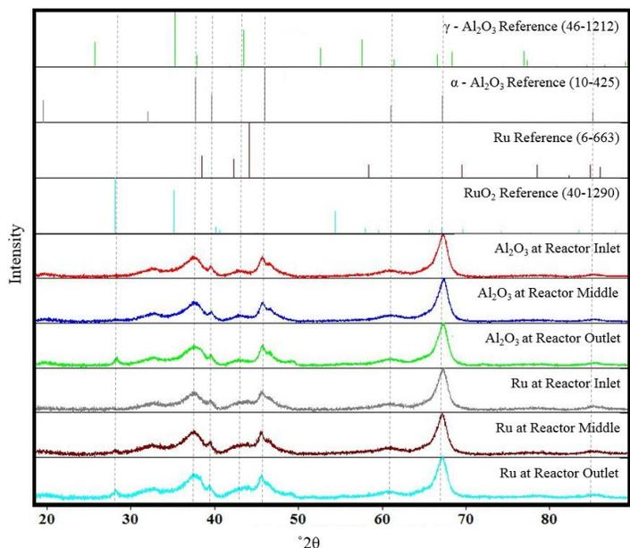
Figure 15. XRD Spectrums of Ru and Al<sub>2</sub>O<sub>3</sub> isolated powders from the pellets from current APM Sabatier reactor.
