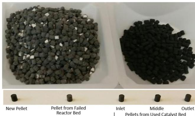
**Figure 4. Top: Left: The 2015/spent catalyst that was damaged; Right: New/unused catalyst; Bottom: Ru/Al<sub>2</sub>O<sub>3</sub> pellets that were characterized.**
