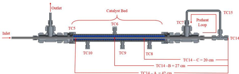
Figure 3. Cross-sectional view of Sabatier reactor model.
