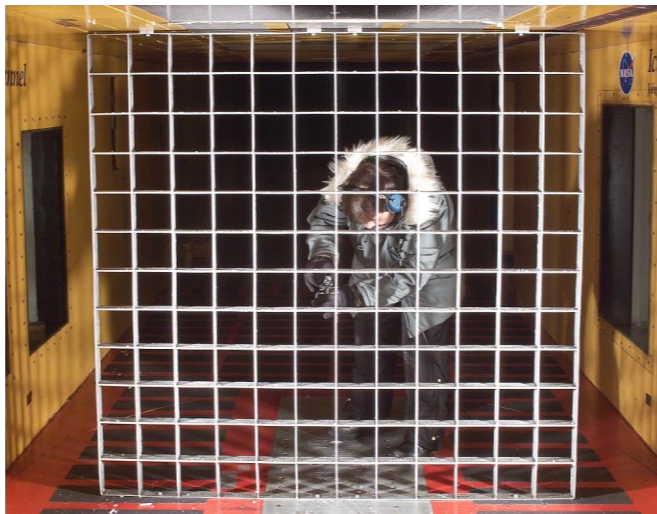
Figure 12. A technician measures the thickness of ice accreted on the Grid.
