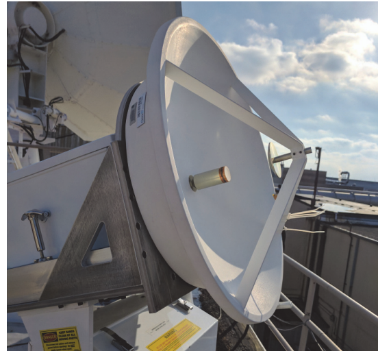
Figure 1. The hybrid beacon receiver and digital radiometer hardware under test at NASA Glenn Research Center in Cleveland, Ohio prior to deployment to the MDSCC in Spain
