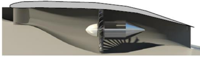
Figure 8: A fan-propulsor housed in the mail-slot nacelle geometry in N3X-DEP.
