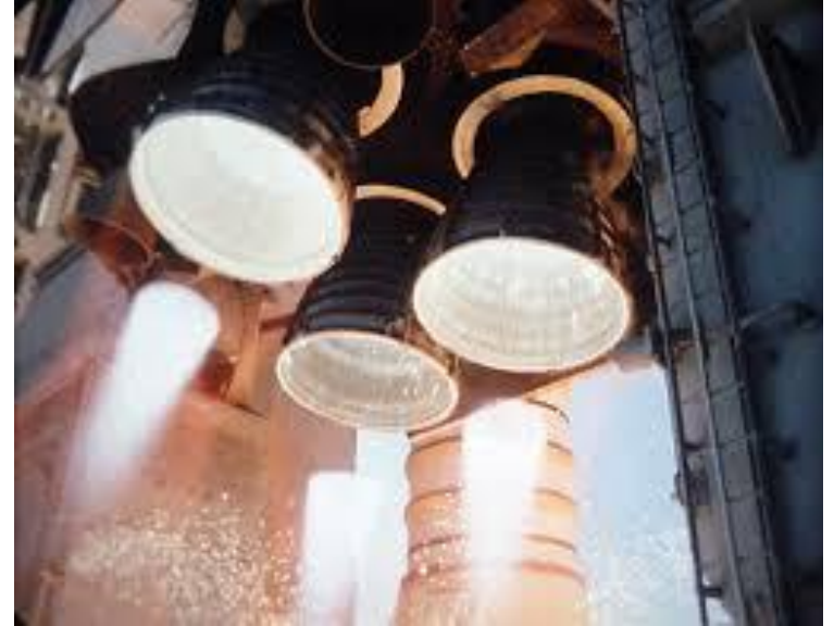
Main Engine Space Shuttle 374,000 lbs thrust (SL) LOX/H 2
