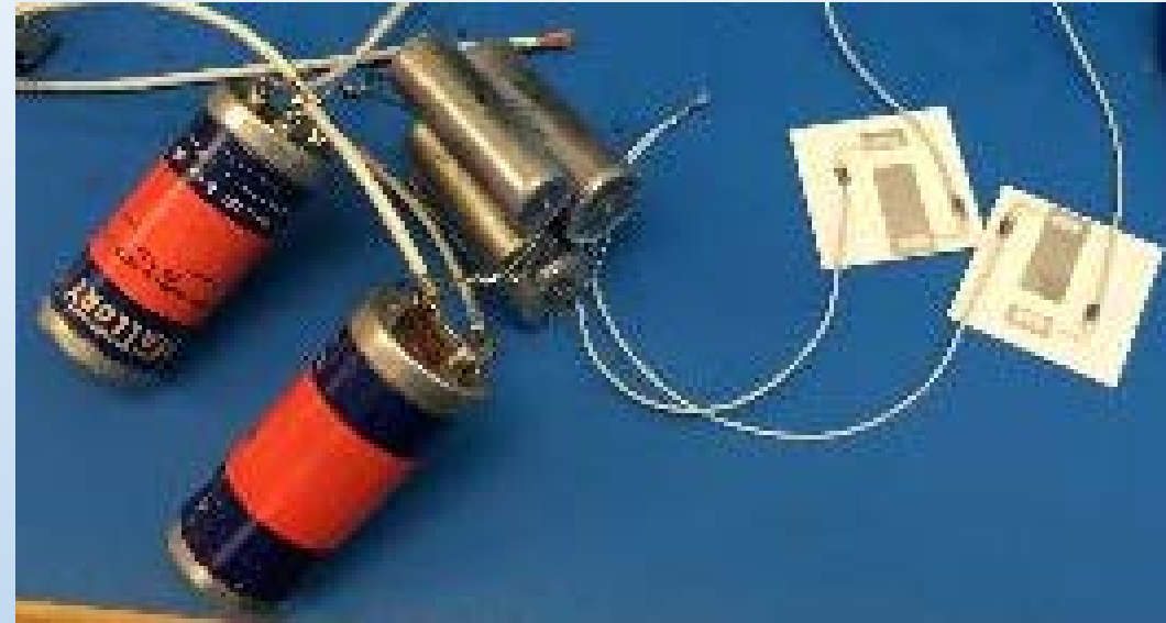
The figure above a capacitor bank beside two single-cell devices manufactured at MSFC. The two ultracapacitors provide the same voltage and capacitance as the capacitor bank. The capacitor bank weighs 435 grams. The two ultracapacitors together weigh only 15 grams with the substrate. The ultracapacitors are only 30 microns thick, 1.8 cm wide and 2.1 cm long
