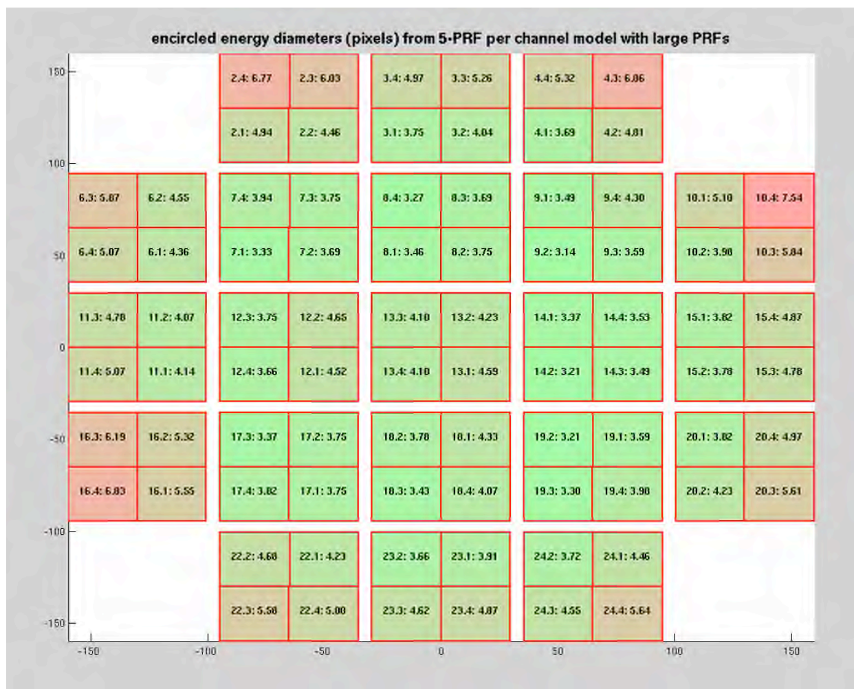
Figure 17: Observed 95% EE diameter after focusing the Kepler telescope (see Bryson et al. 2011 for discussion), arranged in the FPA co-ordinate system. Each box is labeled by channel, followed by the 95% EE diameter in pixels. Green indicates a 95% EE diameter well within the 7.0 pixel requirement, shading to red in those few cases where the requirement is approached or slightly exceeded. The white corners indicate FGS channels.
