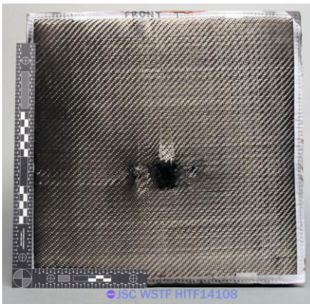
Example of Ballistic Limit Failure Front face sheet damage
