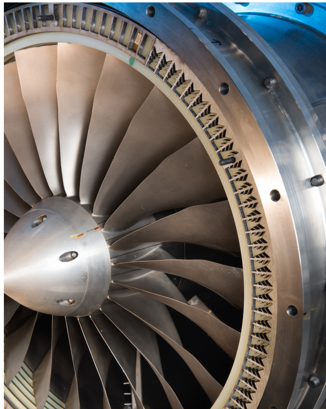
Figure 4: Fan acoustic casing treatment hardware showing the casing grooves, empty chambers and expansion chamber concepts (GRC-2017-C-00942).
