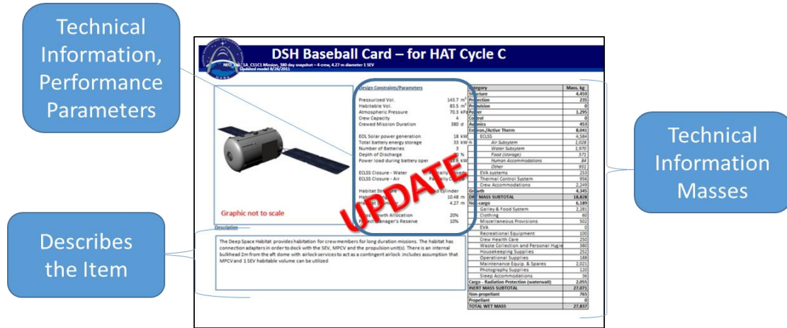
Figure 5. An example traditional space system baseball card focused on technical information. 52 Technical, performance information usually emphasizes mass, plus other characteristics like mission duration or crew capacity. Were this a propulsion stage there would be an emphasis on masses and type of propellant, plus other characteristics like engine thrust or number of engines.
