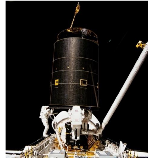
Space Shuttle STS-49 Endeavour Intelsat VI Repair. Astronauts Thuot, Hieb and Akers take manual hold of the satellite as commander Brandenstein delicately maneuvered the orbiter to within a few feet of the 4,215kg communications satellite. Image NASA.
