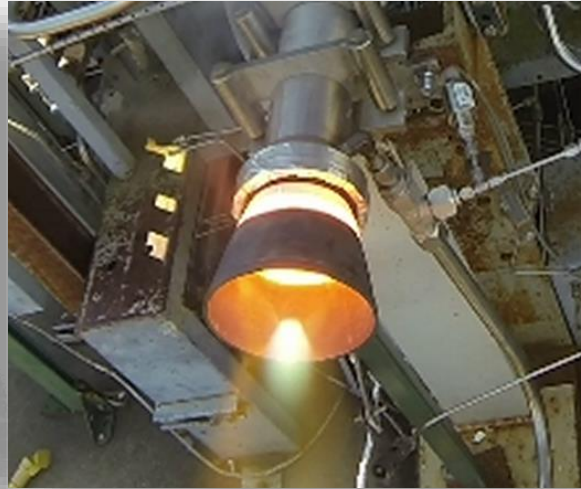
Orbital ATK Extension Test with COIC SiC + Hf
