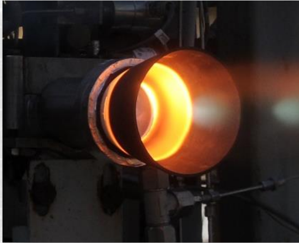
Orbital ATK Extension Test with COIC SiC + Hf
