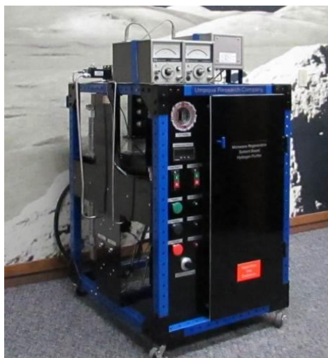
Figure 2. Microwave Regenerative Sorbent-based Hydrogen Purifier (MRSHP).
