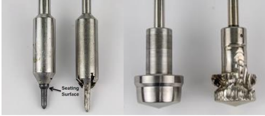
Figure 2: Valve damage due to cavitation of water (Ref 3)
