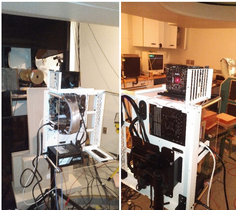
Figure 3: nVidia GTX 1050 GPU in laser alignment beam at MGH
