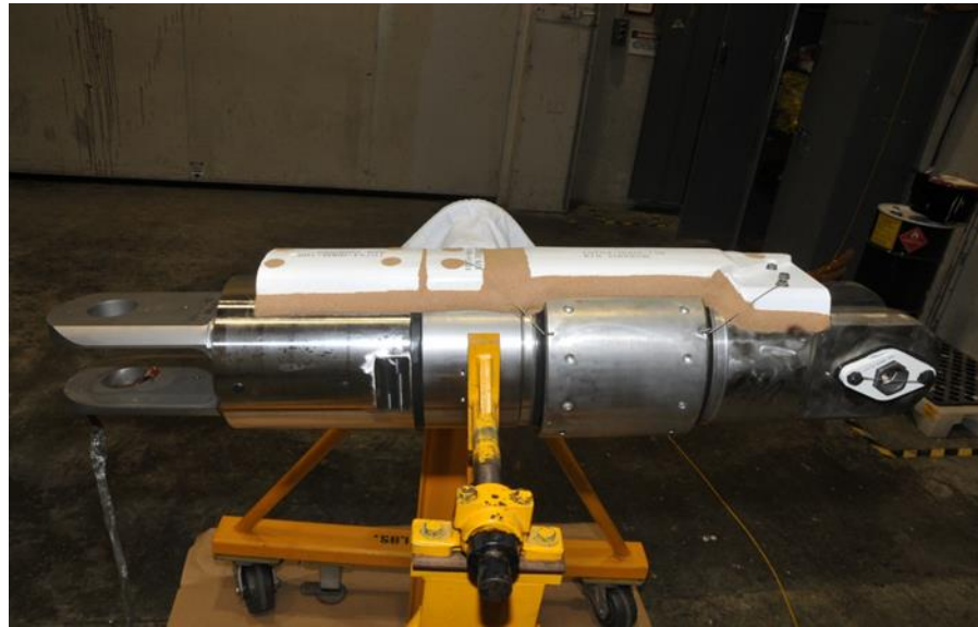
RT-455 closeout on the Diagonal Strut
