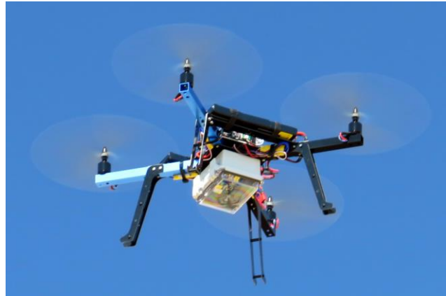
Figure 8. Quadcopter Test Vehicle with Mesh Network Payload
