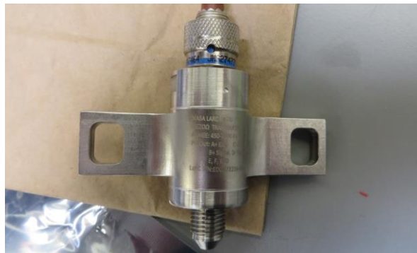
Figure 1. Supersonic pressure transducer developed for MEDLI2.
