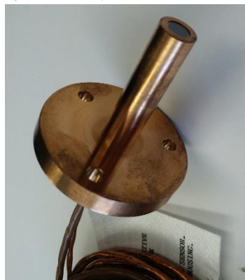
Figure 2. Medtherm radiometer selected for MEDLI2.
