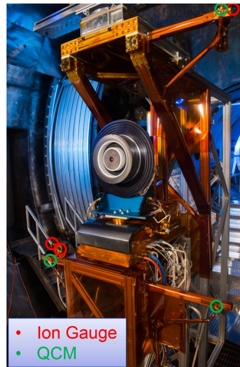
Figure 10. QCM and ion gauge location on the VF-6 test setup.
