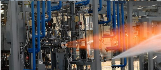
GRCop-84 AM Chamber Accumulated 2365 sec hot-fire time at full power with no issues
