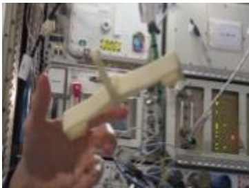
SPHERES Tow Hitch: SPHERES consists of 3 free-flying satellites on-board ISS. Tow hitch joins two of the SPHERES satellites together during flight. Printed 2/21/17.
