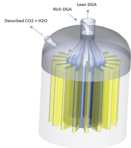
Figure 3: Graphic illustration of capillary driven heat exchanger desorber
