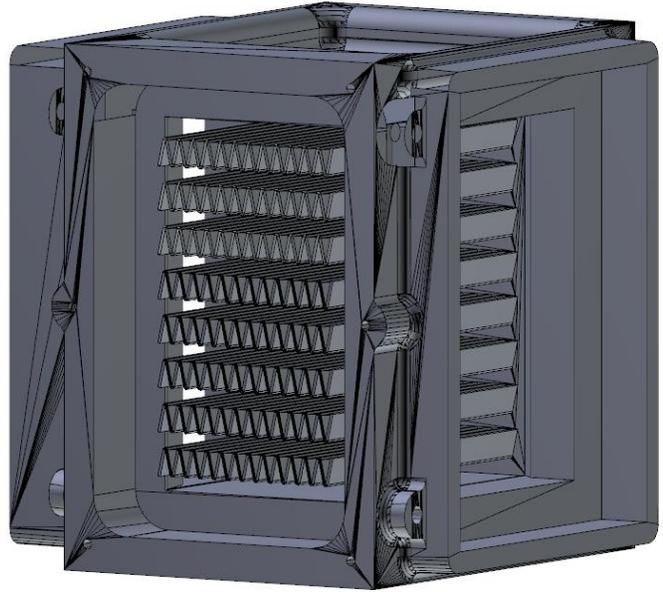
Figure 2: Graphic Illustration of 3D printed direct air/liquid contactor
