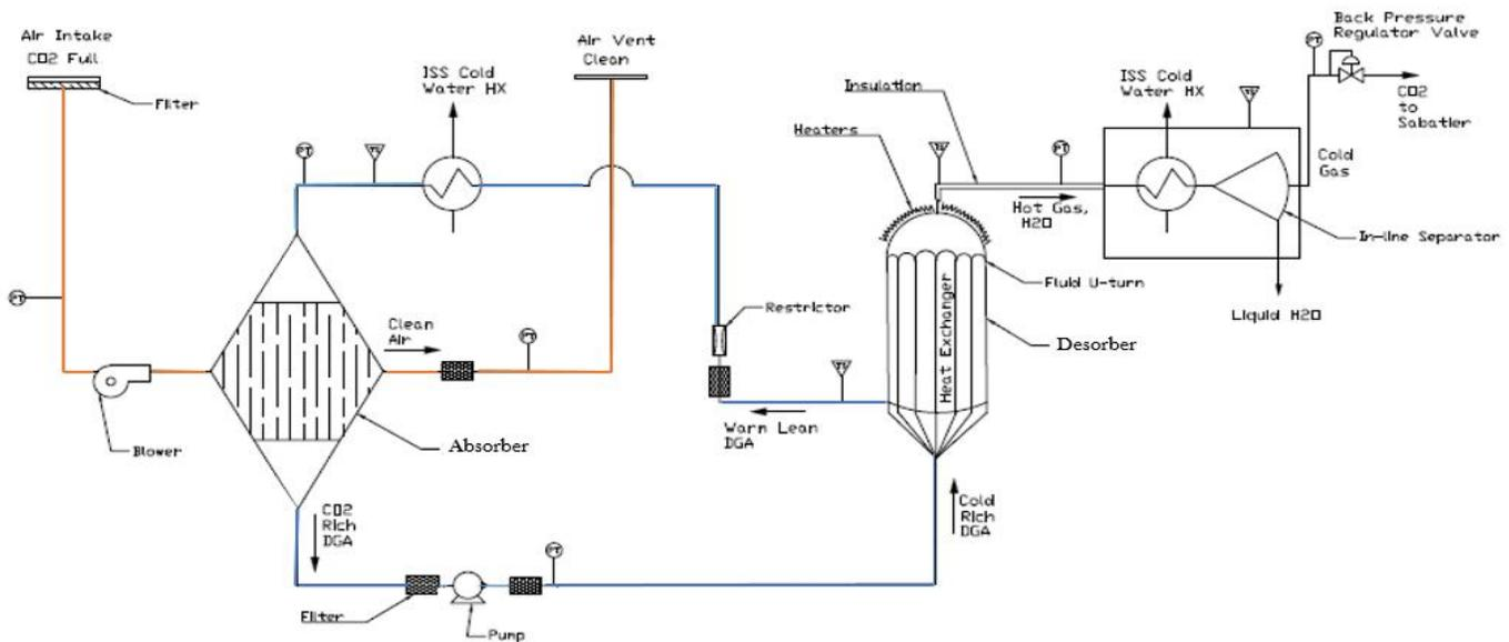
Figure 1: Process and Instrumentation Diagram of LACARS
