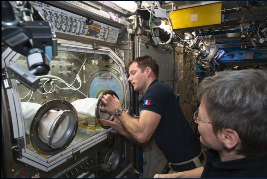
ISS050e042167. Thomas Pesquet (ESA) and Peggy Whitson (NASA) setting up the Microgravity Expanded Stem Cells (MESOC) Life Science Ancillary Hardware (LSAH) in the Microgravity Science Glovebox (MSG).
