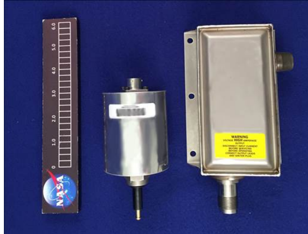
Figure 5: Exciter units tested with ASI igniter Compact-style unit (left); Conventional-style unit (right, without lead) In both units, the spark igniter connection is at the bottom
