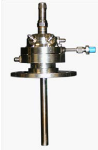
Figure 3: MSFC ASI igniter body
