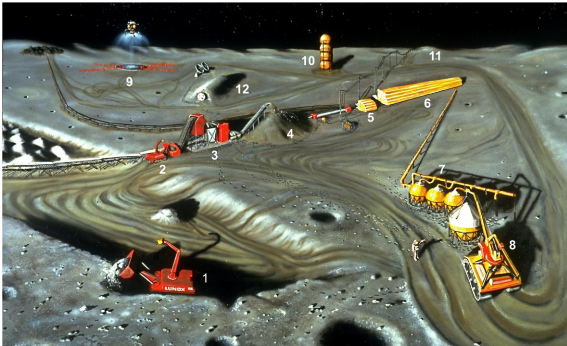
Figure 4. Activities at a LUNOX Production Plant Processing Ilmenite-bearing Feedstock Materials (ca. 1983)
