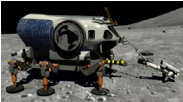
Figure 1 Simulation screen capture showing PEV with hopper system and astronaut on an APS.
