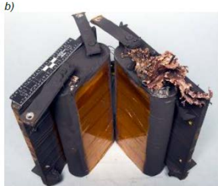
Figure 1.2-2. After test imagery of HITF12143 a) shield with 9.5cm diameter through-hole, and b) cell close-up with impacted cell on right showing molten material from cell interior that was ejected and deposited on exterior of cell.
