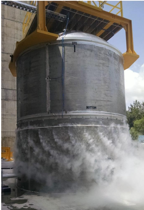
Fig. 27. Chilling the test stand with liquid nitrogen.
