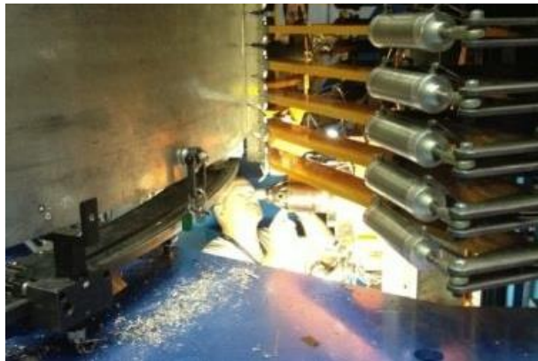
Fig. 14. Dynetics barrel on the Vertical Weld Tool.
