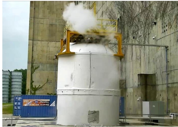
Fig. 29. Integrated test article is chilled down with liquid nitrogen (shows boiloff at top of tank).
