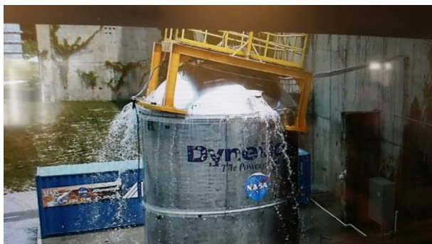
Fig. 33. Several seconds after tank burst.
