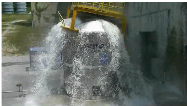
Fig. 32. Several seconds after tank burst.
