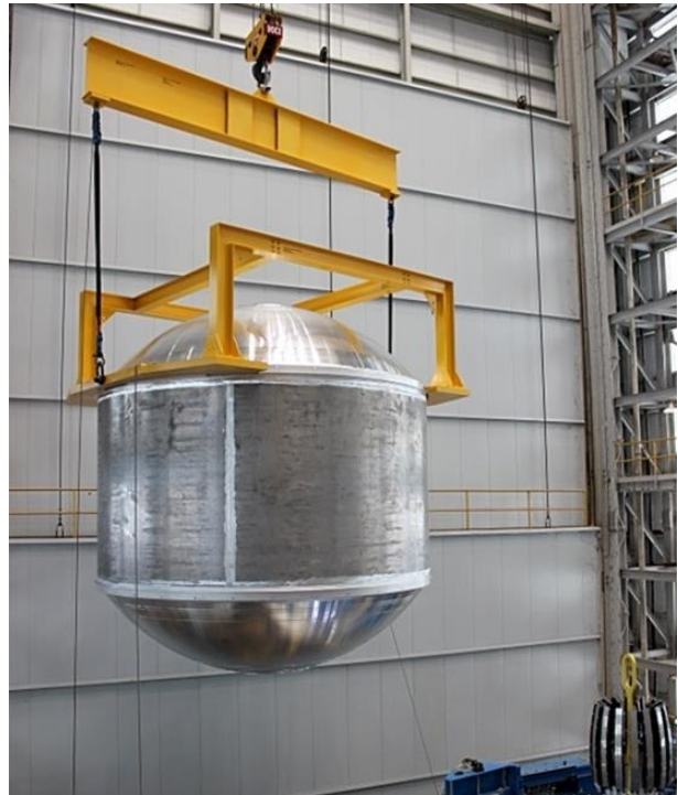
Fig. 19. Completed tank removal From VAT using forward lifting fixture.
