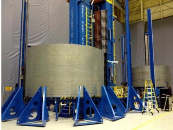
Fig. 13. Dynetics barrels on MSFC FSW tools, Vertical Weld Tool (near) and Vertical Trim Tool (far).
