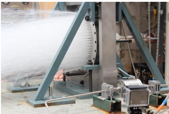
Fig. 8. F-1B SLM GG injector flow calibration test.
