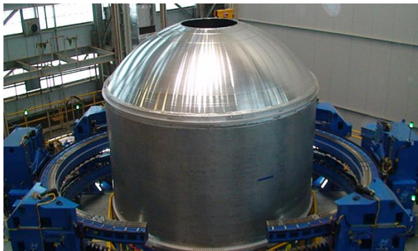
Fig. 18. Forward weld completed on tank in VAT.
