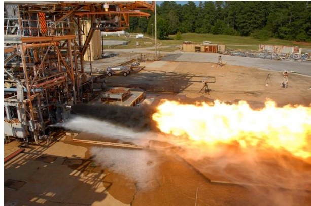
Fig. 9. F-1B SLM GG injector hotfire test at MSFC.
