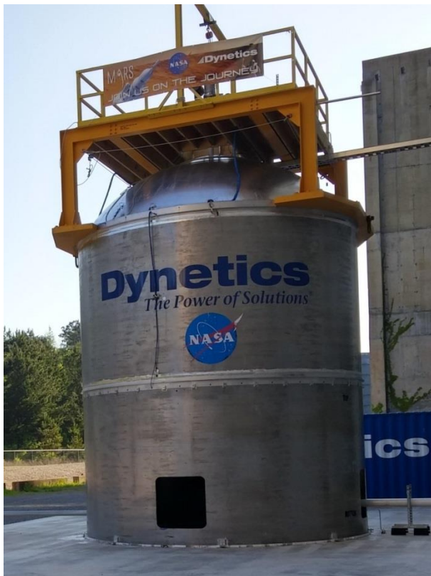
Fig. 26. Integrated test article on the test pad.
