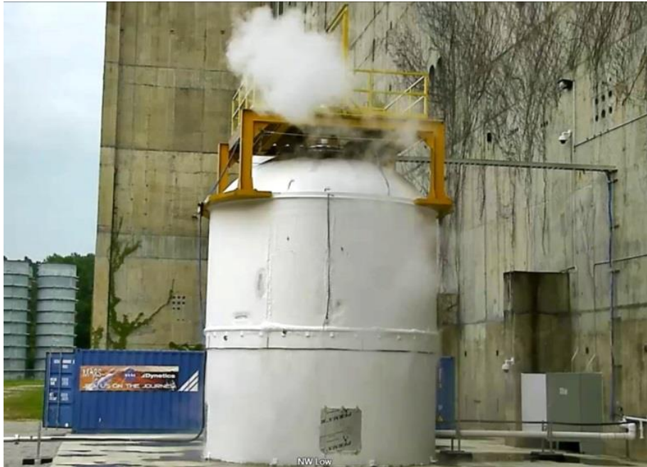
Integrated test article chilled with LN_2
