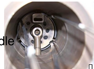
Injector and turbulator modified for CMC liner integration and testing
