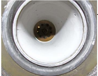
First set SiC/SiC liner Thermocouple (TC) arrangement configurations (total 24 TCs, 1/16" size), film cooled liner planned for second and third set testing
