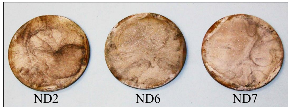
High pressure burner rig tested new ND series Hybrid EBC systems coated on 2" diameter Gen II Prepreg SiC/SiC CMCs
