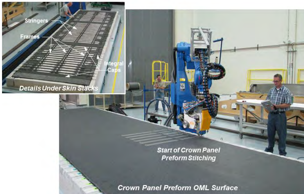
Figure 5-7. Initial Seam Laydown on First Panel Stitched (Crown Panel)
