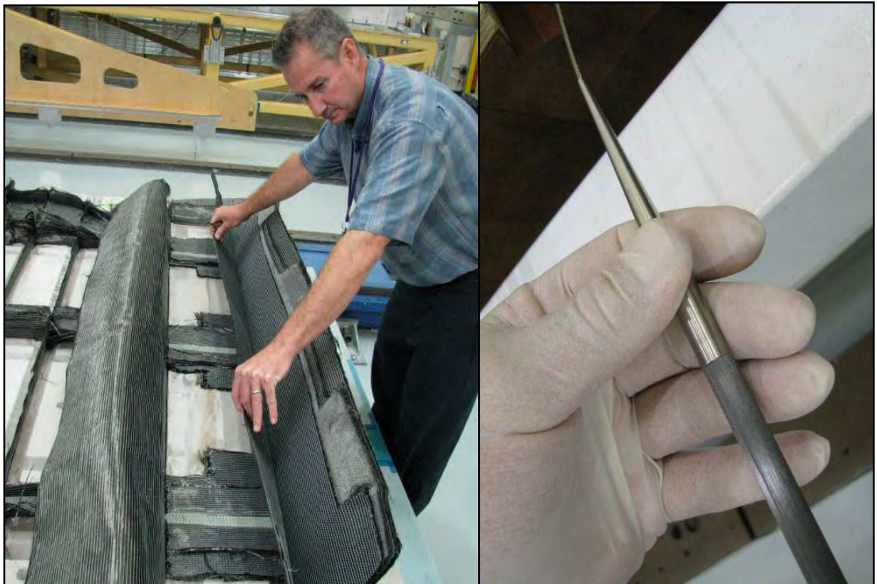
Figure 6-11. Forming of Cap and Frame Flanges (left), Carbon Rod With Leader Wire Adapter (right)
