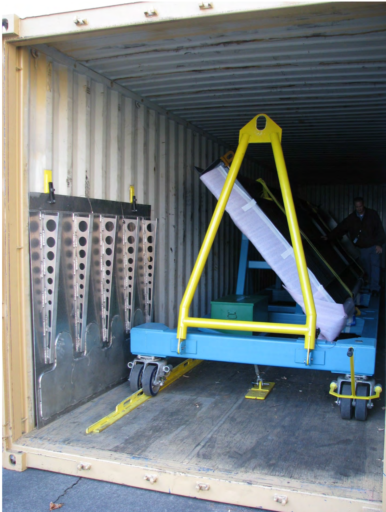
Figure 6-30. Panel on Transportation Dolly Loaded Inside SEAVAN Container
