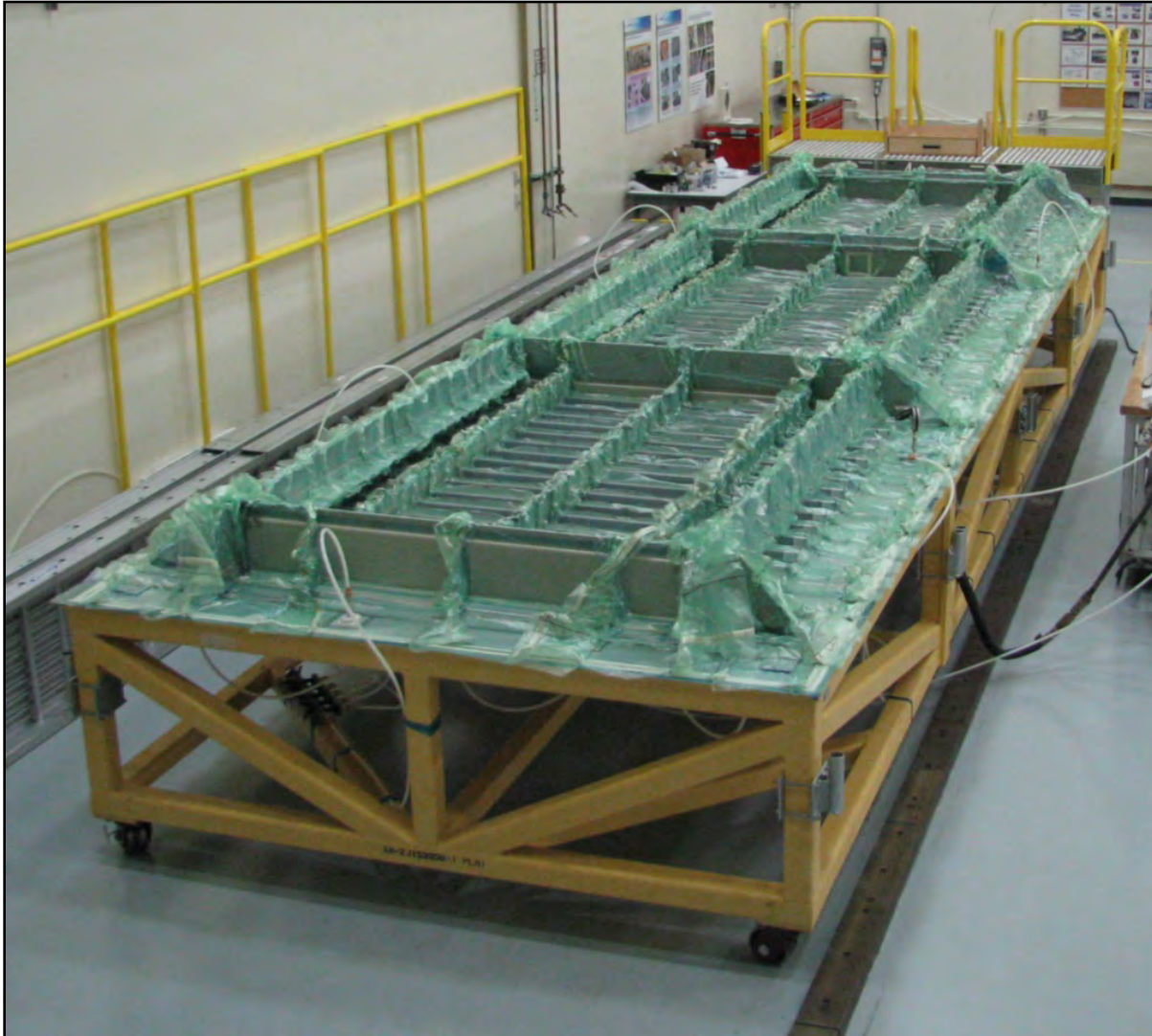
Figure 6-18. Installation of Vacuum Bag Over Crown Panel Preform and IML Tooling
