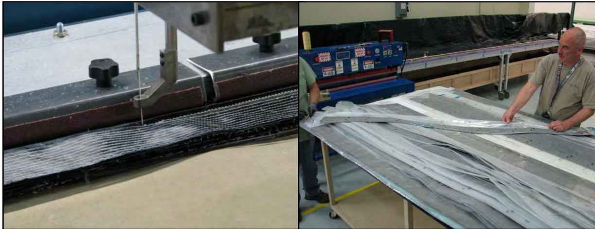
Figure 6-5. Stitching of Stringer Preform Web Shown With Vacuum-Bagged Stringer Preforms
