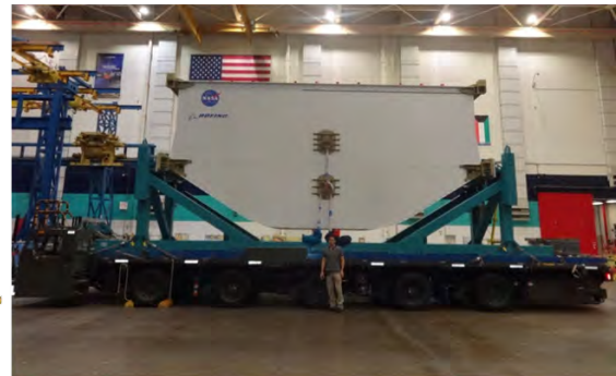
Figure 6-121. Loading the MBB on the K-Loader for Loading Onto the Super Guppy
