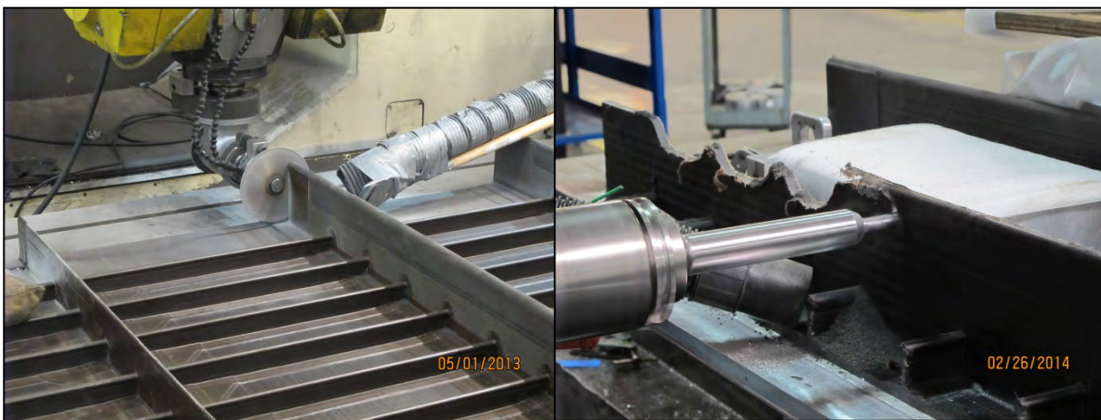
Figure 6-32. Machining of Center Keel Panel Periphery and Bulkhead Cap Web
