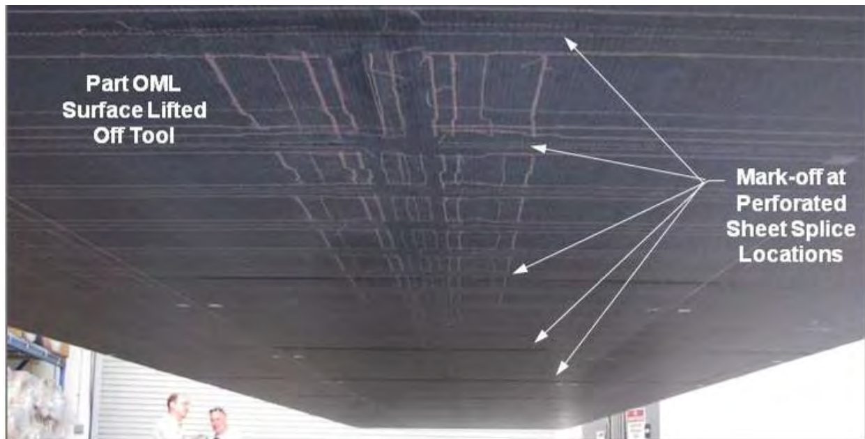
Figure B-1. Thermal Expansion of Caul Sheets Caused Mark-off on the Crown Panel OML
