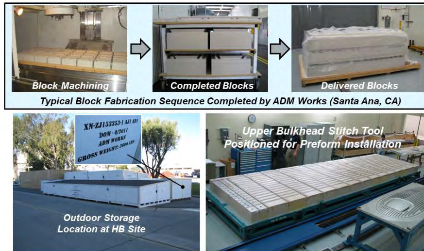
Figure 5-4. Foam Block Fabrication and End Use on Stitching Table
