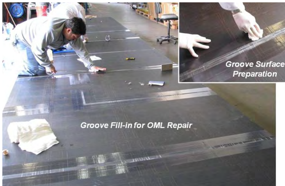
Figure B-10. Crown Panel OML Surface Prepared for Repair
