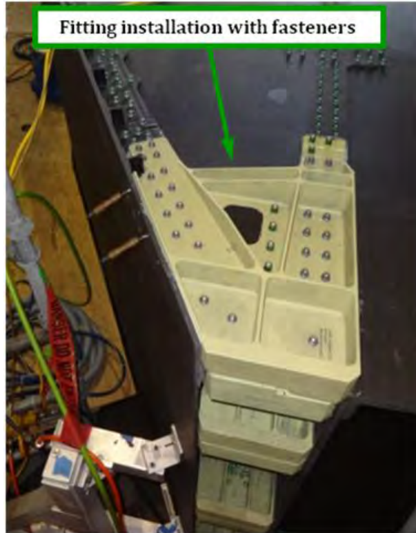
Figure 6-55. Typical Fitting With Completed Fastener Installation
