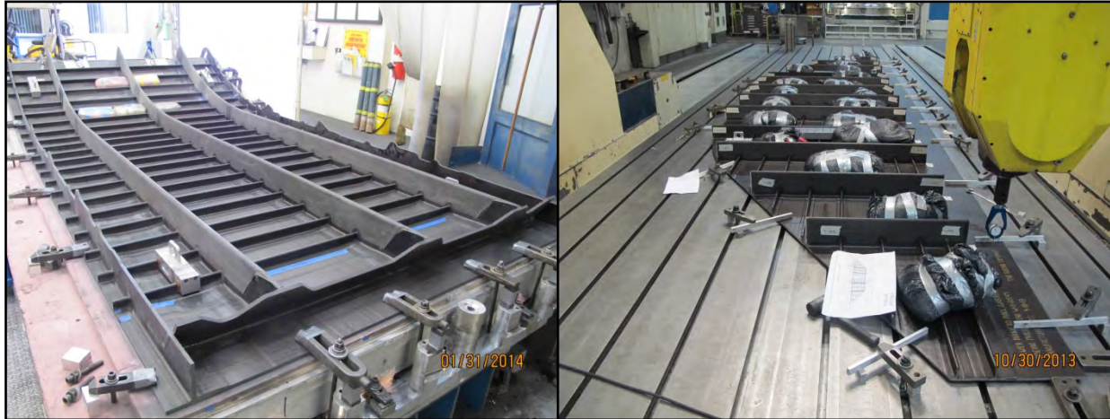
Figure 6-31. Periphery Machining of Lower Bulkhead Panel (left) and Side Keel Panel (right)
