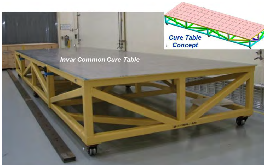
Figure 5-9. Common Cure Table Used to Support Different IML Tooling Arrangements
