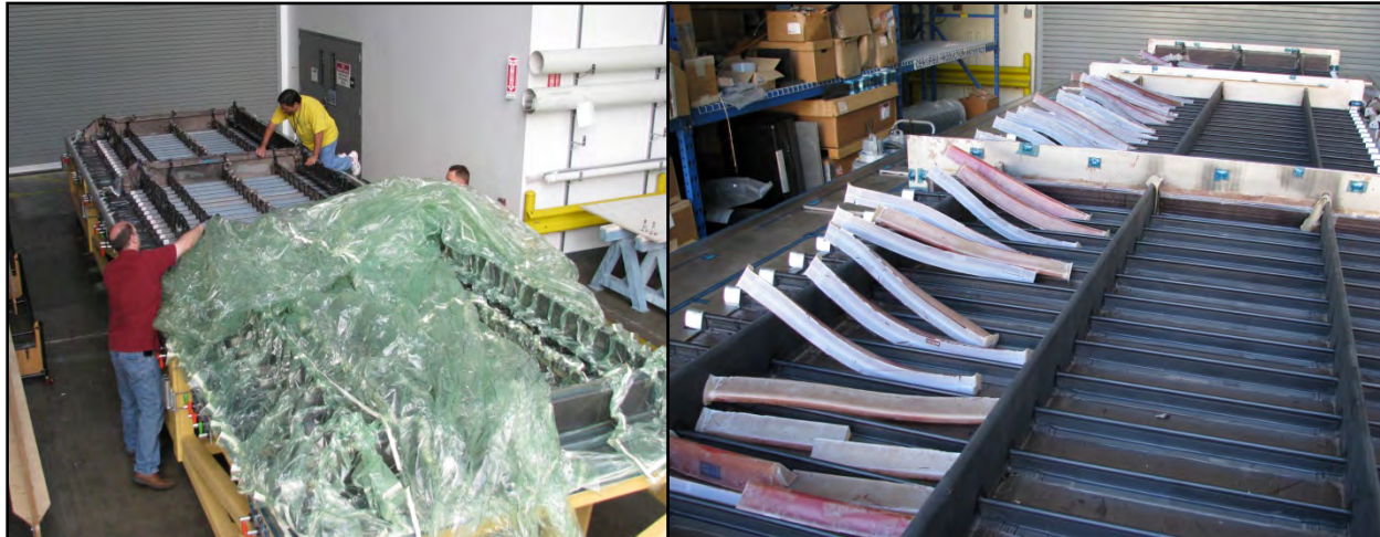
Figure 6-21. Removal of Vacuum Bag and IML Tooling From Infused and Cured Panel
