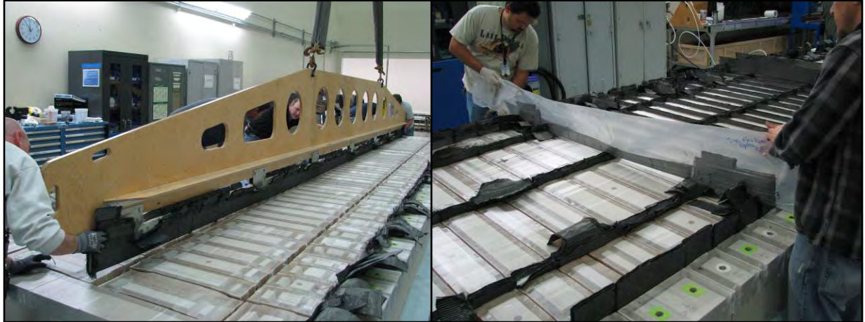
Figure 6-10. Installation of Frame (left) and Stringer (right) Preform Details Into Assembly Jig
