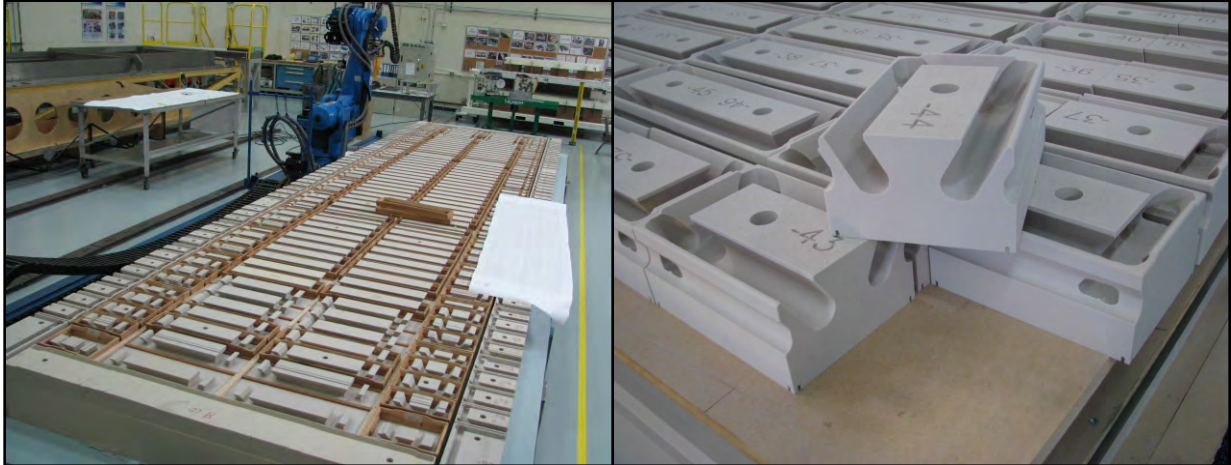
Figure 6-9. Preform Assembly Jig for Crown Panel Utilized Machined Foam IML Tool Blocks
