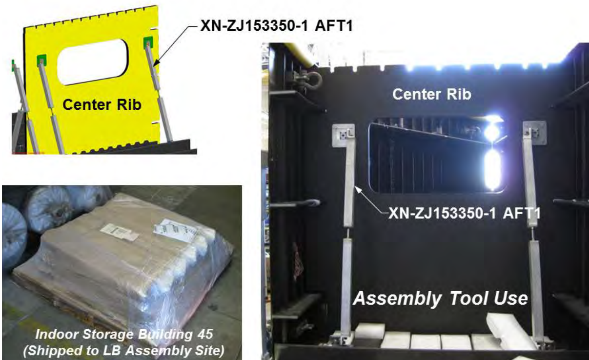
Figure 5-17. Holding Aids Used to Support Internal Ribs During Assembly
