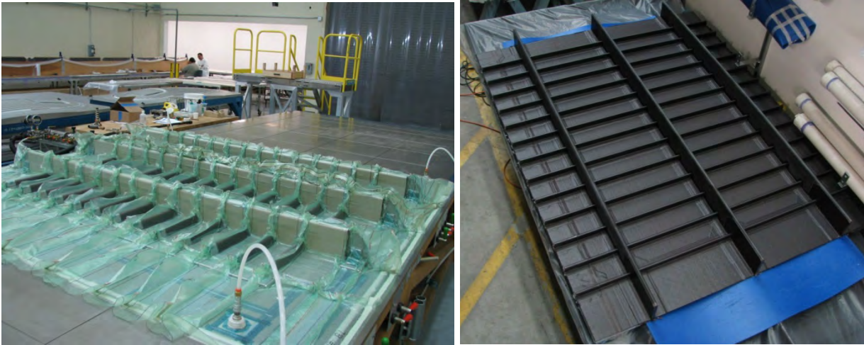
Figure 5-14. Rib Panel Shown Under Vacuum Before Infusion and After Cure
