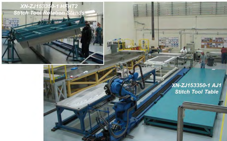
Figure 5-3. Common Stitching Table Used to Support Different Foam Block Configurations
