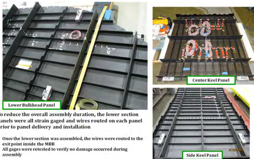
Figure 6-72. Lower Panels Were Strain-Gaged Before Assembly
