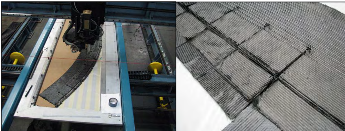
Figure 6-6. Stitching of Bulkhead Cap Preform Shown With Net-Size Features
