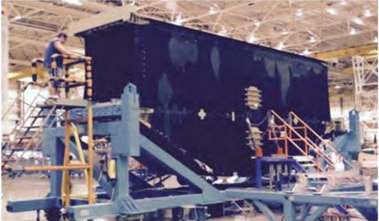
Figure 6-75. MBB Leak Check at 6 psi Using Soapy Water to Detect Leaks
