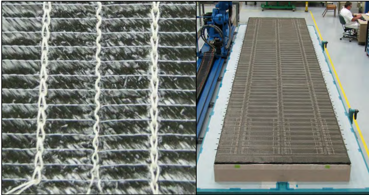
Figure 6-14. Modified 3D Chain-Stitch Seam (left) and Complete Crown Panel Stitching (right)
