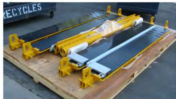
Bar Members and Panel Lift Plates
