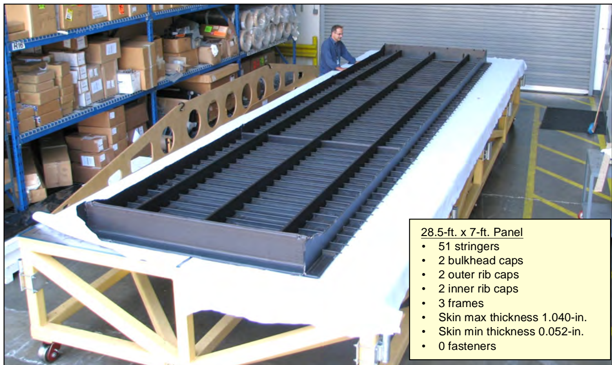
Figure 6-22. Resin-Infused and Cured Crown Panel Before Periphery Machining
