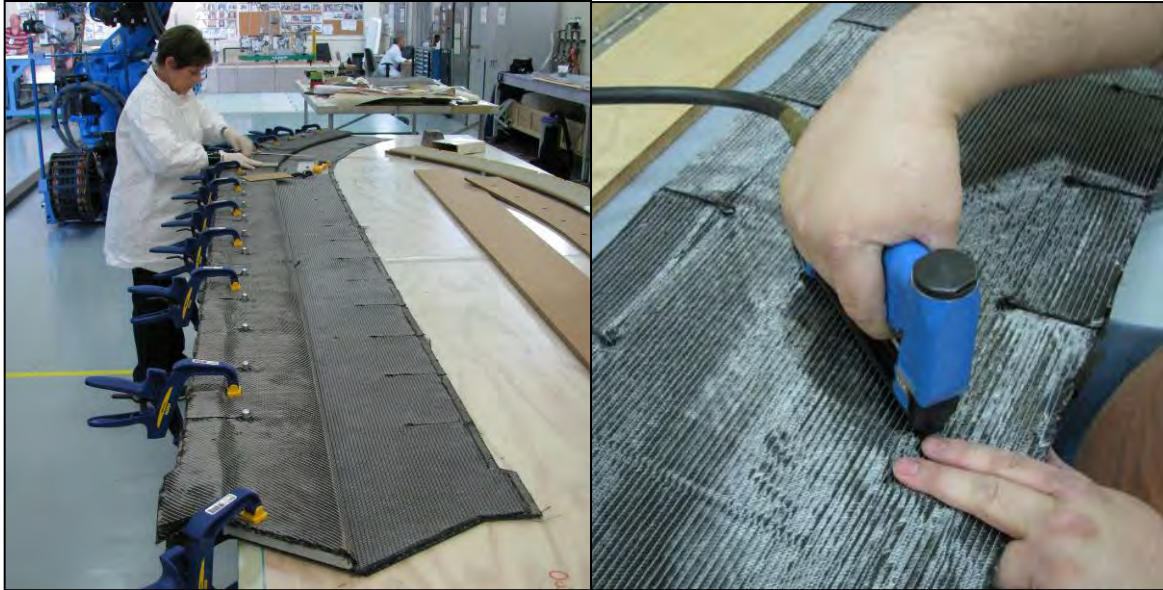
Figure 6-8. Layout and Subsequent Stapling of Fabric to Foam Core for Frame Component
