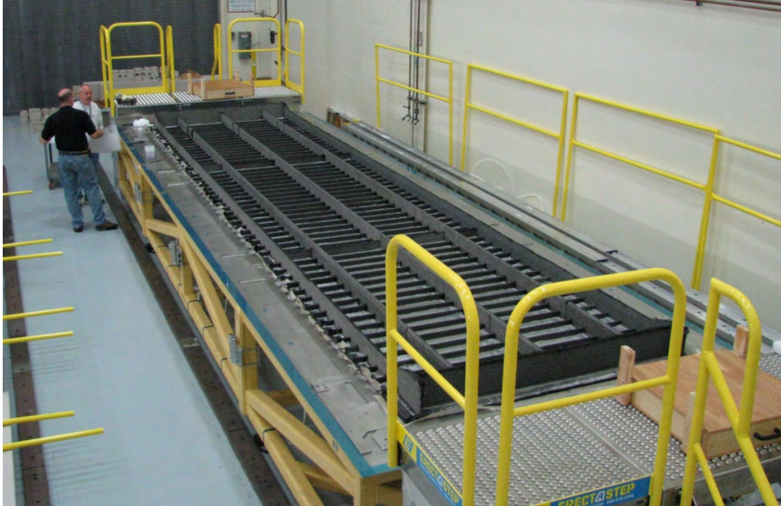
Figure 6-16. Crown Panel Preform Positioned on OML Tool
