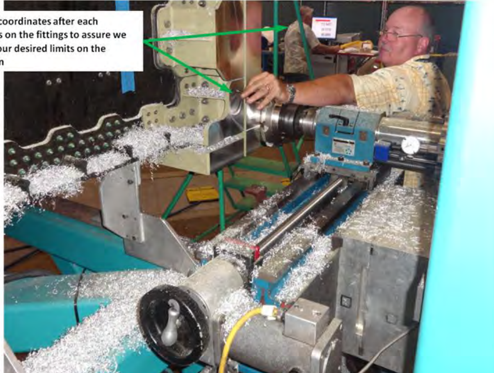
Figure 6-61. Milling the Load-Introduction Fittings—Checking X, Y, and Z Coordinates
