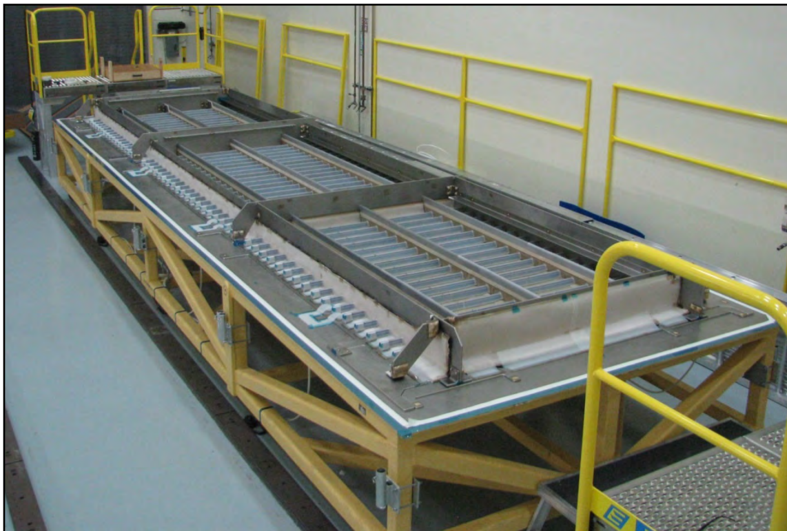
Figure 6-17. Installation of IML Tooling Over Crown Panel Preform
