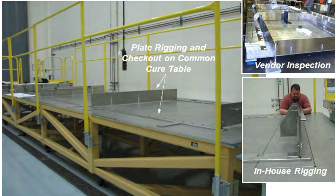
Figure 5-10. IML Details Rigged and Checked Out on Common Cure Table
