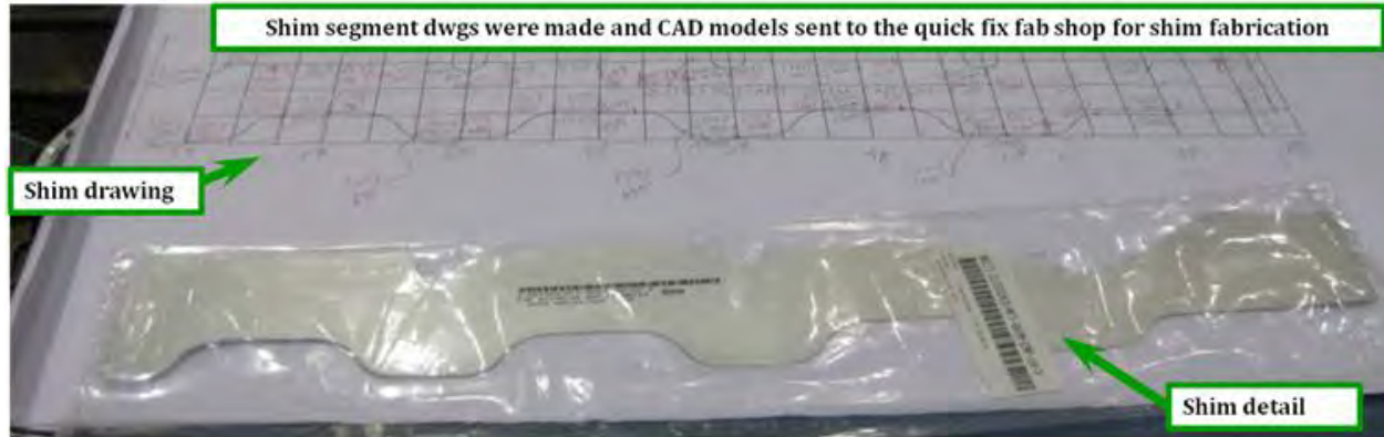
Figure 6-42. Typical Shim Drawing and Fabricated Shim Detail
