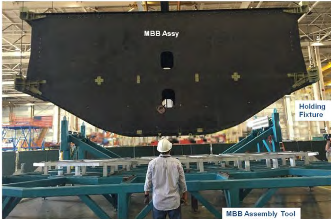
Figure 6-69. Multi-bay Box Assembly Moving Into the Holding Fixture
