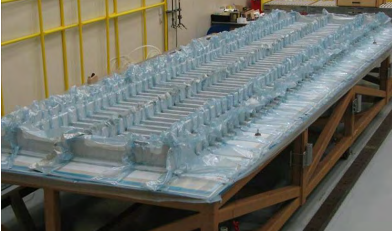
Figure B-13. Bagged Crown Panel With IML Side Facing Up and Repair Patches Taped to the OML
