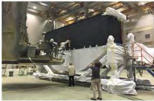
Painting the Lower section of the MBB
