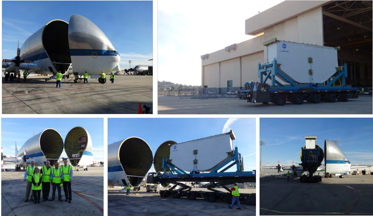
Figure 6-123. K-Loader Loading the MBB Into the Aircraft
