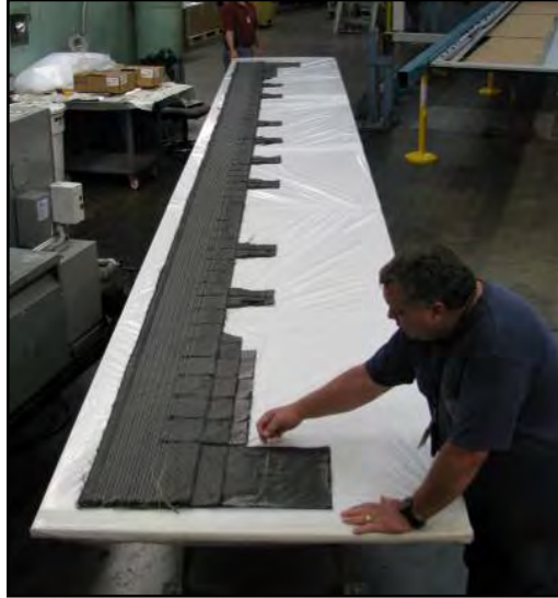
Figure 6-7. Complete Bulkhead Cap Preform for Crown Panel With Extended Flange Stacks
