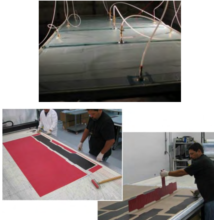
Figure B-9. Patches Were Infused and Cured in an Oven and then Secondarily Bonded
