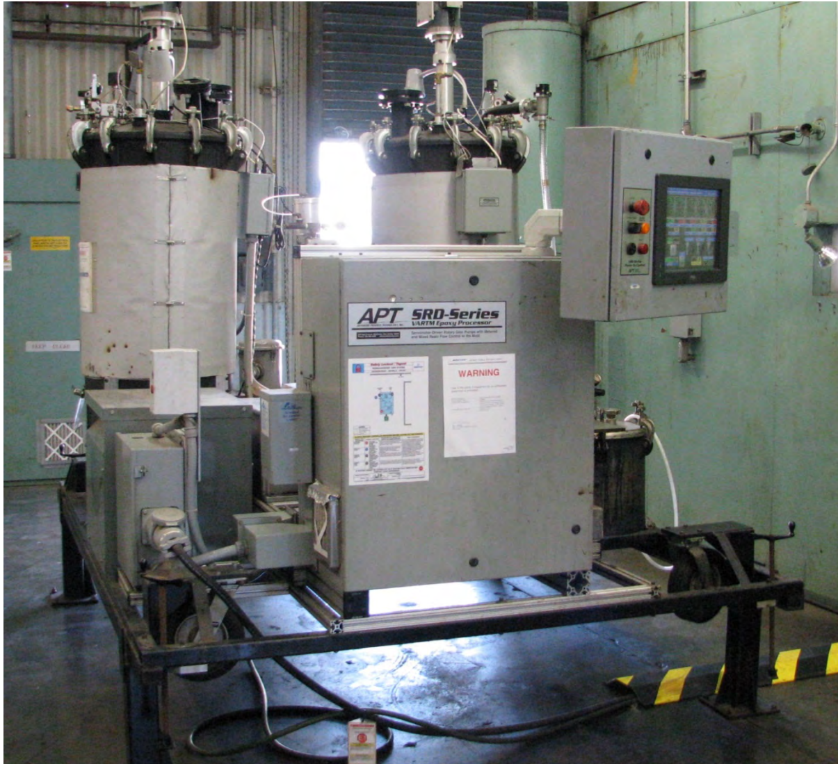
Figure 6-19. APT Servo Rotary Dispensing Machine for Automated Resin-Infusion Processing
