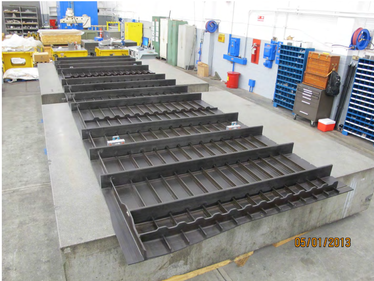
Figure 6-33. Upper Bulkhead Panel Positioned on Surface Table for Final Dimensional Inspection
