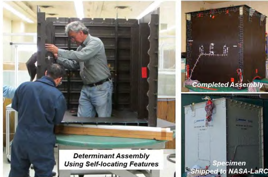
Figure 2-9. Cube Test Article Used to Validate MBB Design Approach
