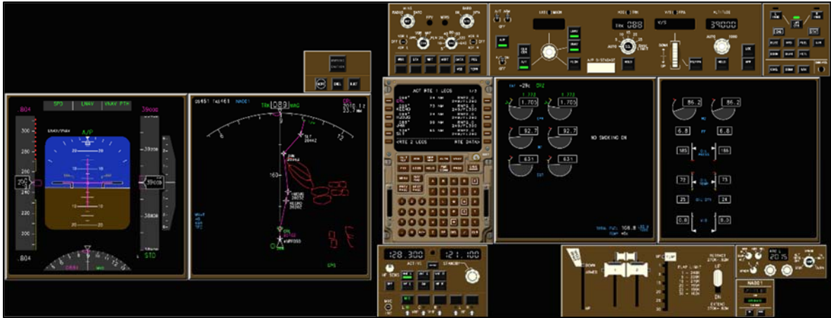
Figure 12. ASTOR Simulation with the RPFMS CDU Shown at the Center of the Image.
