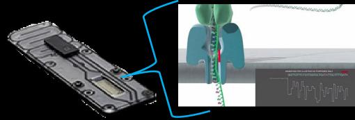
Flow Cell: Contains the nanopore sensing technology that is required to perform the sequencing reaction
