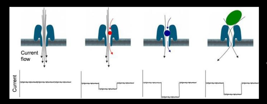
Nanopore-based sequencers measure changes in current caused by DNA strands migrating through the pore. The changes in current are characteristic of the sequence of migrating DNA.
