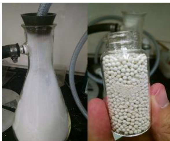
Figure 10. Physical Sorbent Degradation Experiments. The left image was taken during the vacuuming of sorbent from a large beaker into the flask. The zeolite dust coats the inside of the flask, hose, and vacuum line. The right image is a sample removed from the larger volume of sorbent after it has been poured back into a large beaker. Visible chips of sorbent created by the violent nature of the vacuuming process are shown.
