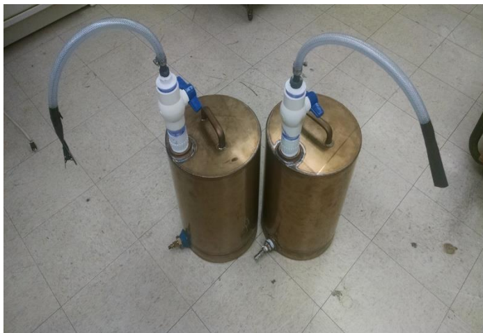
Figure 1: Custom CRCS Bakeout Canisters. These canisters were designed to aid in activating the CRCS sorbent material.
