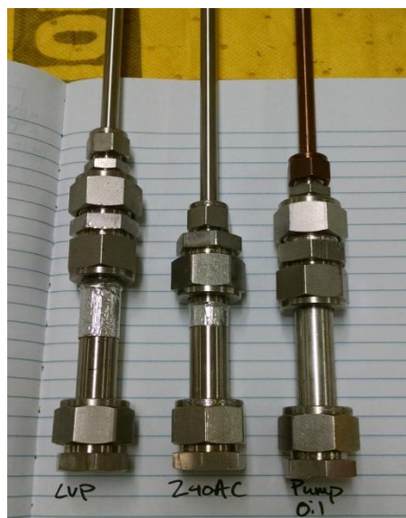
Figure 5: Chemical contamination cells. These cells are filled with Stage 1 sorbent and suspected contaminants – Krytox LVP, 240AC, and Edwards Ultra Grade 19 vacuum pump oil.
