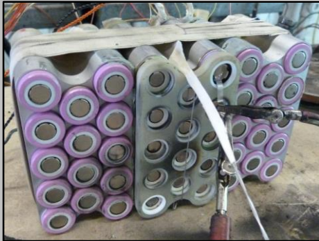
JSC Test Unit With Interstitial Barrier and Heat Spreader (Design Template)
