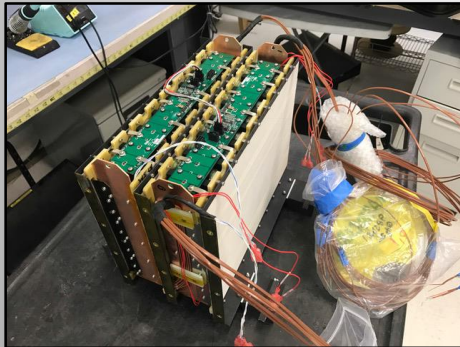
X-57 Thermal Runaway Unit (2 Trays; ½ Module)
