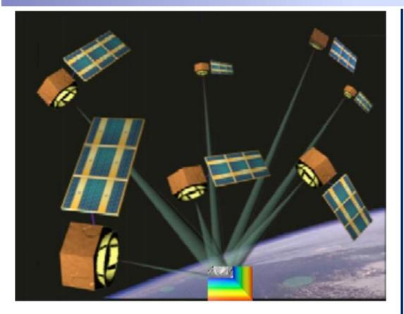
A satellite formation making multi-angular, multi-spectral measurements by pointing its spectrometers at the same ground spot, as it orbits the Earth (not to scale).
