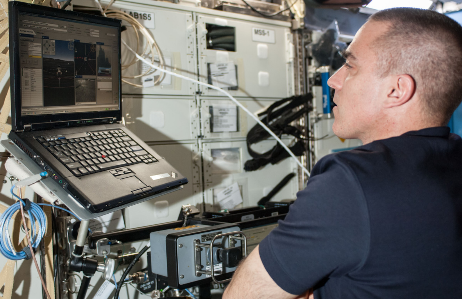
Chris Cassidy uses the “Surface Telerobotics Workbench” to remotely operate K10 from the ISS
