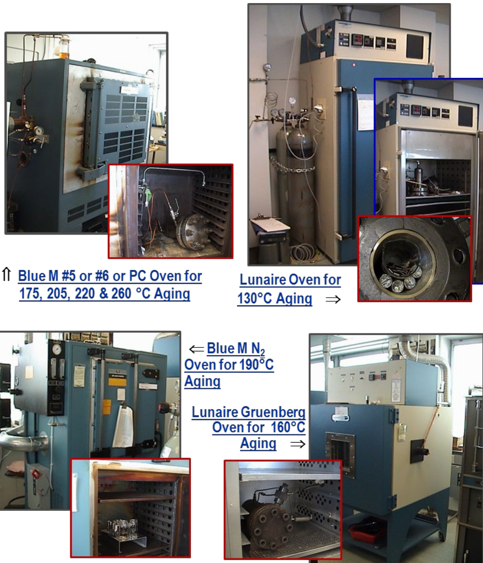
Figure 12.—Various ovens and pressure vessel systems equipped with dry nitrogen gas flow control used for thermal aging experiment.
