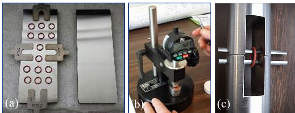
Figure 11.—(a) O-ring compression-set test setup, (b) Type M Durometer for o-ring hardness, and (c) Fixture for o-ring tensile test.
