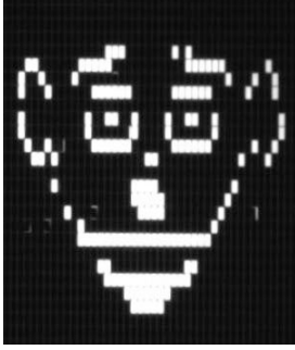
Fig. 5: A photo of the microshutters selectively opened with a back illumination.
