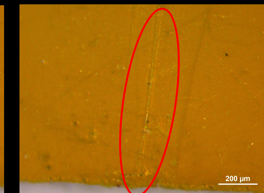
Kapton HN/VDA sample after being bend tested to 4.49% surface strain. Bend test induced crack is highlight with the red circle.
