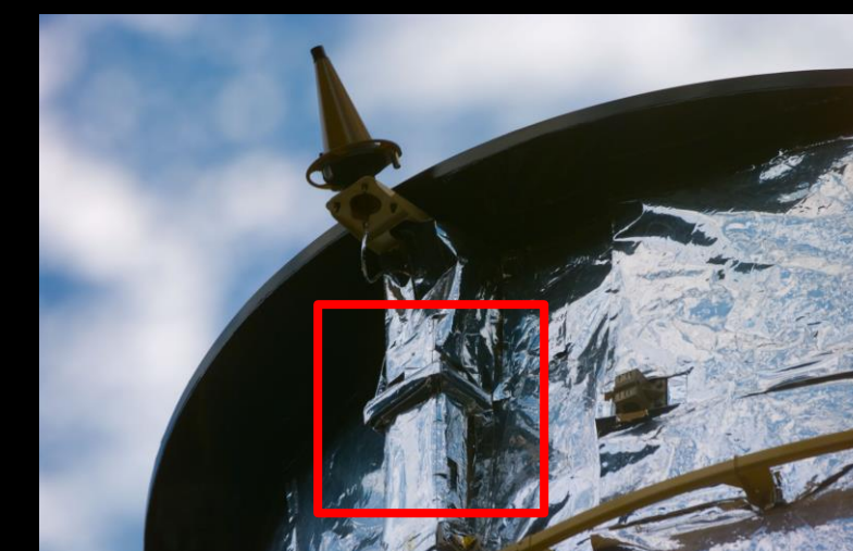
Spacecraft blanket wrapped about a corner on the HST
