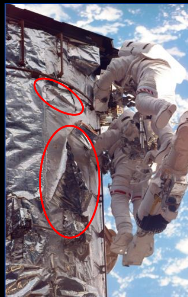
Radiation induced embrittlement & cracking of Teflon insulation (6.8 years in space)
