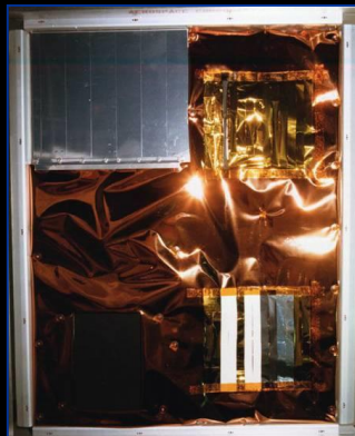
AO erosion of Kapton blanket
