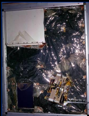
AO erosion of Kapton blanket
