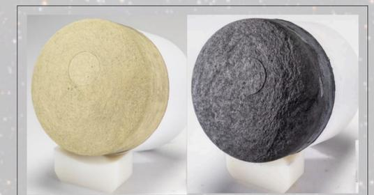
PICA before & after arc jet testing
