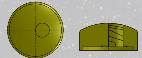
4" diameter Iso-q arc jet model with plug
