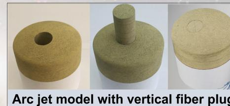
Arc jet model with vertical fiber plug
