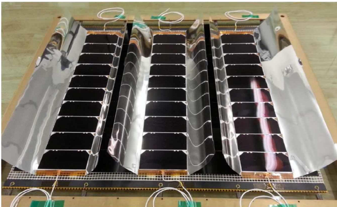
Figure 2: Concentrator equipped power module
