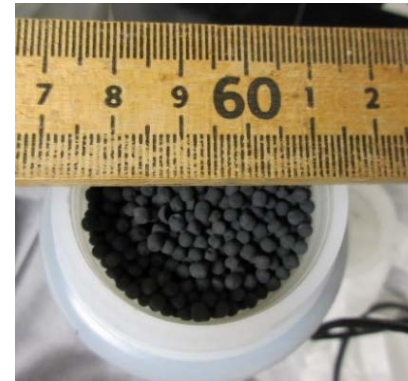
Packed bed material for ISS WRS, Catalytic Oxidation Reactor (Alumina or Zirconium beads)
